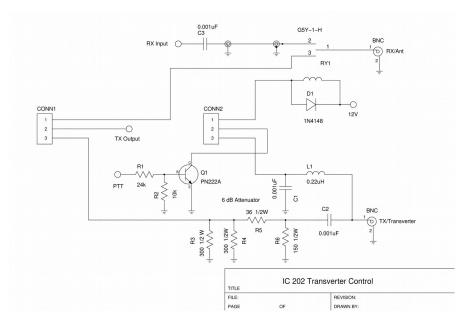
Figure 4: Transverter control circuit.
