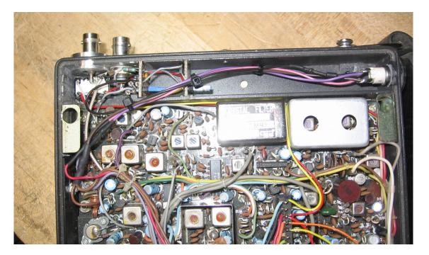
Figure 5: T/R relay and transverter circuitry. The relay is in the far upper left corner.
