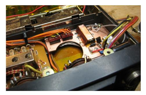
Figure 2: Display board under the speaker. The PIC in the upper right center is covered with Kapton and copper foil tape to reduce computer hash. The TCXO is the white object to the right. The LO junction terminal is just to the upper right of the PIC. The white wire visible on the wafer switch in the front goes to the MOSFET gate.
