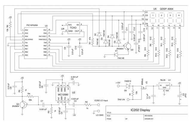
Figure 1: Display circuit
