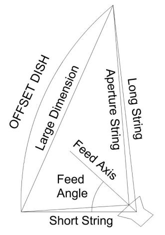
Figure 4 – String lengths to align with center of aperture
