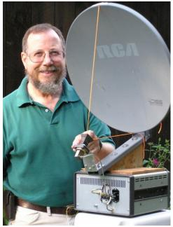
Figure 2 – Finding dish focus using string method
