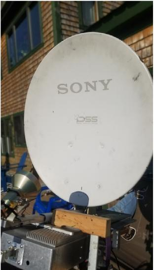
An additional advantage to sun noise is that the difference between measured elevation tilt on the digital level and the known sun elevation tells you exactly how far to tilt the offset dish to be on the horizon.
