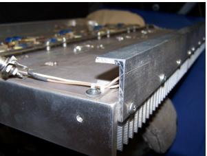
Aluminum channel stock is used for the side rails. Size is ¾ X 1 ½ X 1/8" wall. (This picture is of a 4 FET amp)
