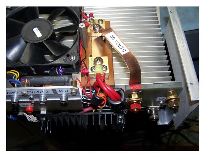
Close up view of the home brew 100 amp shunt and the fiberglass DC input panel. I used 5/16" brass hardware. The negative terminal is directly grounded to part of the aluminum chassis, while the positive lead runs over to the shunt. The big red wire and ferrite donuts attach to the FET DC switch mounted on the black heat sink that extends behind the main chassis/ heat sink.
