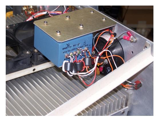
OP-AMP METER DRIVER BOARD in an RF proof enclosure is mounted on the front panel near the power meter. There are two multi turn potentiometers inside the enclosure that adjust forward and reflected power through two access holes. Note the front panel side brace.
