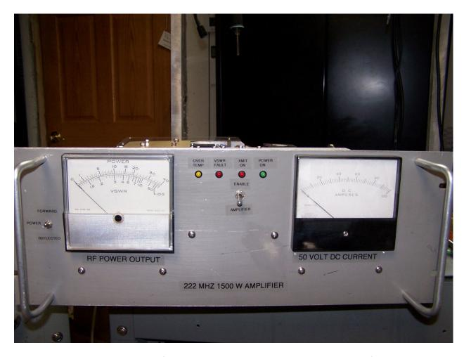
Front panel view of the converted 1500 watt Larcan 222 MHz amplifier
