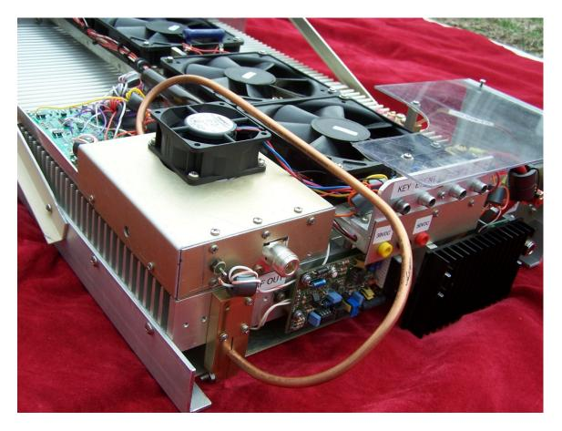
This is the final version of the amplifier with a metal enclosure over the output filter. Note the cooling fan to keep the filter components cool. It is a small 24 VDC fan with a 500 ohm dropping resistor from the 50 volt buss to limit noise but still provide adequate cooling for the filter coils.
