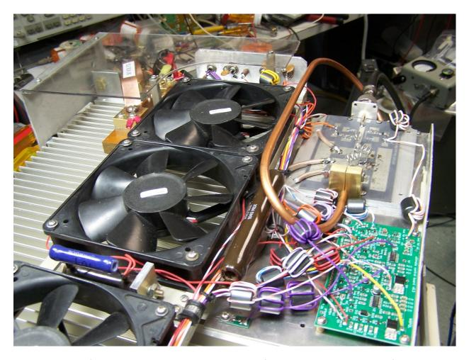
A detailed view of the W6PQL Control Board. I wired all of the connections to the top of the board. I also used some mix 43 toroids on all of the connecting leads to control any RFI problems. For best results at 222 MHz, use no more than three turns of wire on each toroid.
