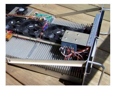
Another view of side rails along with the front panel braces. I used 1/8" aluminum angle bracket material. Panel braces are needed to properly support the 1/8" thick aluminum front panel.
