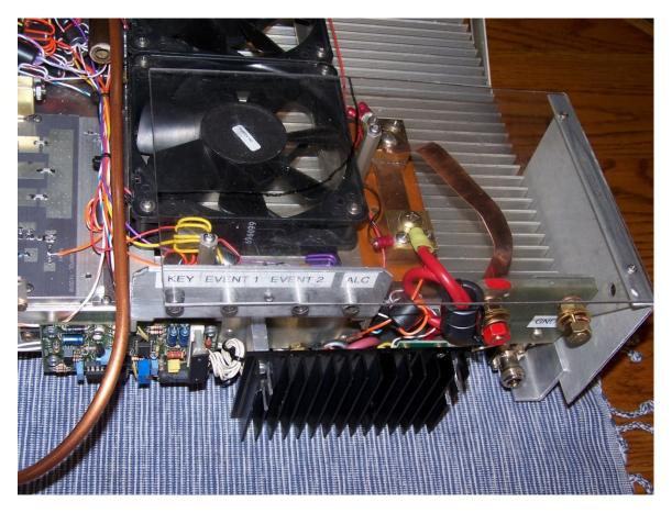
Here is the right rear portion of the amplifier. The Larcan protection board is on the left. The black heat sink in the middle contains the FET DC switch. The 50 volt power terminals are on the far right.
