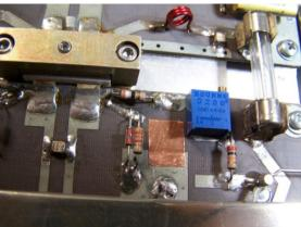
A View of the bias circuit of the four FET 222 MHz Larcan amplifier. The yellow polyester cap on the left photo is the only bias bypass capacitor and it has rather long leads especially for 222 MHz. The 0.50" X 0.35" copper foil addition can be seen in the right photo all ready to accept the two chip cap bypass caps. NOTE THAT THESE CHANGES ARE NOT NEEDED IN THE LARGER SIX FET AMPLIFIERS.
