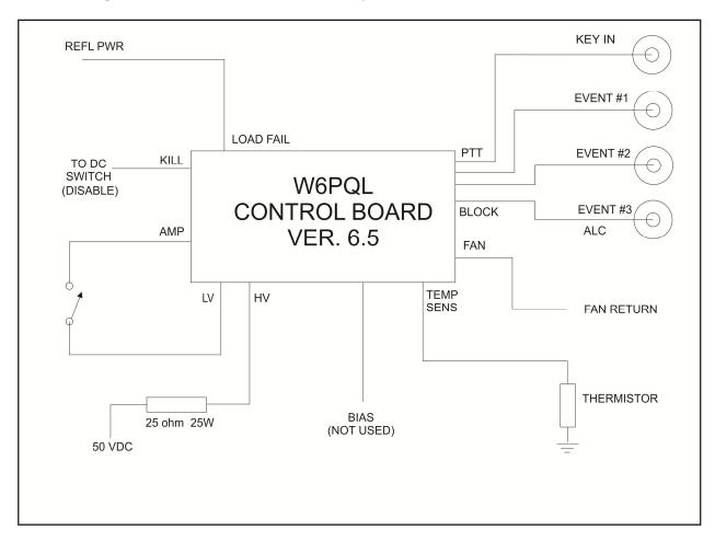
Wiring diagram for Version 6.5 of the W6PQL Amplifier Control Board. The switch shown between the LV & AMP terminals must be included to connect 12 vdc to the "AMP" pad on the board.
