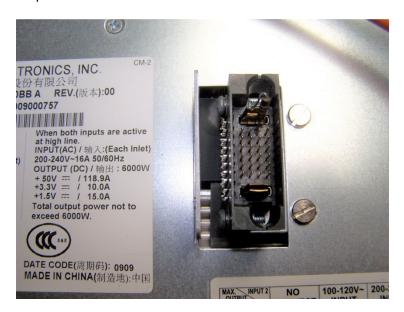
Cisco DPST 6000BB Power Supply. "ENABLE" connections to activate the 50 volt output. Connect 3<sup>rd</sup> pin from left on top right (as shown) to the adjacent large blade connector pin with a 500 to 1K resistor.
