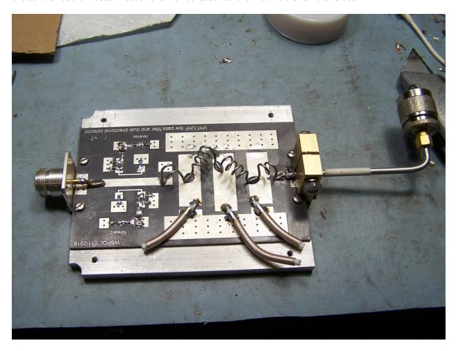
The W6PQL 222 MHz Filter modified for high power. Substrate is some ¼" aluminum plate. The chip caps have been replaced by short lengths of Teflon coax. This particular filter measured -48 dB at the 2<sup>nd</sup> harmonic, and -60 dB at the 3<sup>rd</sup> harmonic frequency. Return loss through the filter is over 30 dB.
