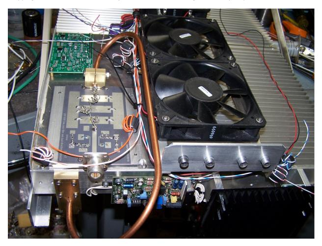
This is a photo of the back of the amplifier while under construction. The RF filter board sits on top of the main heat sink. The W6PQL Control Board is seen in the back ground just behind the RF filter.
