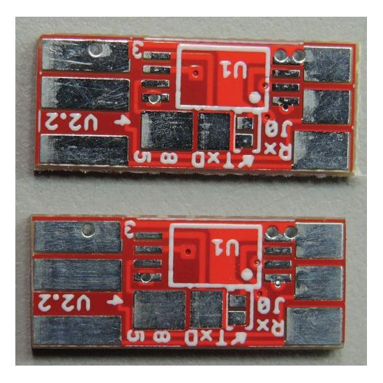
Populate all the components on both sides of the PCB. As the PCB is small, there wasn't room to provide identification for all components on the silk screen, so use the PCB top and bottom layouts below to identify part locations. The PCB top side has three Mini DIN solder pads. The bottom has two.
