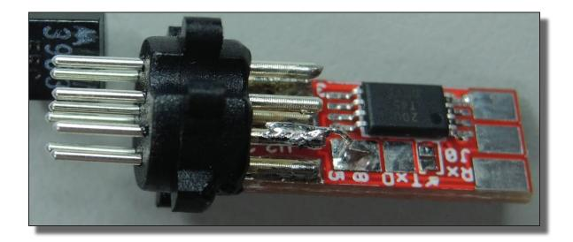
Wire soldered from SP8 to Mini DIN pin 8
