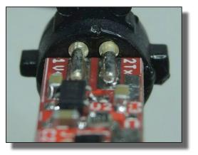
isn't much room for misalignment. Adjust the PCB location if necessary to make sure it fits within the Mini DIN's metal surround casing.
