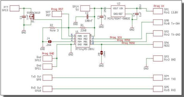
Mini DIN Sequencer V2.2 Circuit Schematic
