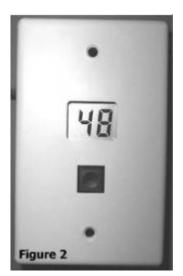
The indicator unit, in Figure 2, is a simple two-digit readout with a pushbutton which turns it on for a minute or so. It may be powered by an internal 9-volt battery or an external 12 volt supply. A four-wire cable connects the two units together; the cable supplied might be long enough for an RV, but I added some cheap rotor cable to reach up the tower.
