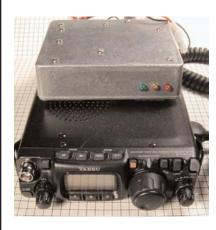
Description One of my projects the previous winter was a "Miniverter" - a barebones printed-circuit transverter for 144 MHz. My intent was to install these inside small 10meter transceivers to make microwave IF rigs. Then I was seduced by the FT-817 - but the Miniverter became the start of a 222 MHz transverter.
