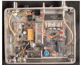
ing. The schematic diagram includes not only plenty of capacitors, but also different values at different frequencies - the values are chosen for operation just below the self-resonant frequency of each capacitor. The power amplifier, A7, is bypassed for a wide frequency range, shown in the detail photo in Figure 6, since bipolar transistor amplifiers are prone to oscillate at low frequencies. Chip capacitors are small enough to use freely, and inexpensive enough, perhaps
