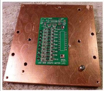
One thing I did notice is that my temperature profile was a bit too aggressive. Some of the resistors show signs of excessive heating. Testing them shows they are electrically fine, but it means my temperature sensor in the oven is not really close enough to reflect actual board temperature. I have edited the temperature profile on the RefloLeo SD card to lower the overall curve. We'll see how the next boards come out.
