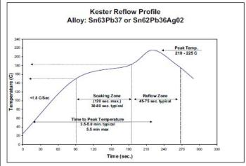
The RefloLeo controller has several user temperature profiles stored on its SD card. I used the standard profile as it looked to be a good match for the Kester Profile. The profiles stored on the RefloLeo SD card are simple text files that are easy to edit.
