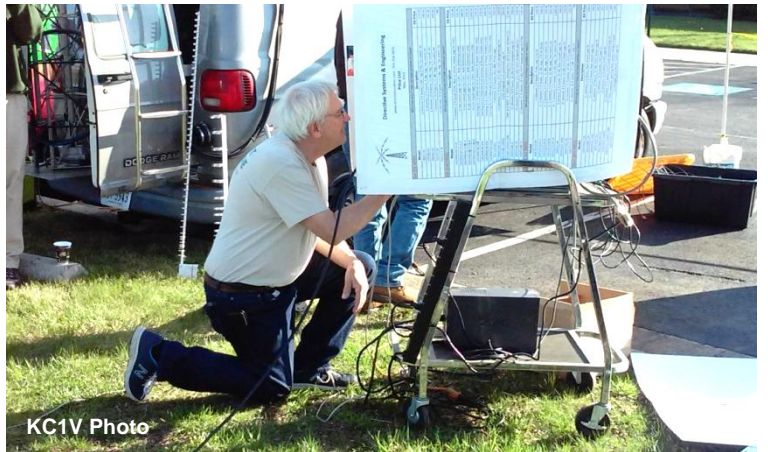
K1WHS making antenna measurements with the network analyzer. The poster board shields the screen from the bright sunshine.
