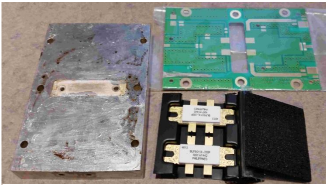
Fig. 1 - NXP BLF6G13L-250P Evaluation board
