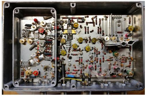
Figure 1 - Inside Microwave Modules 432-MHz SSB Transverter
