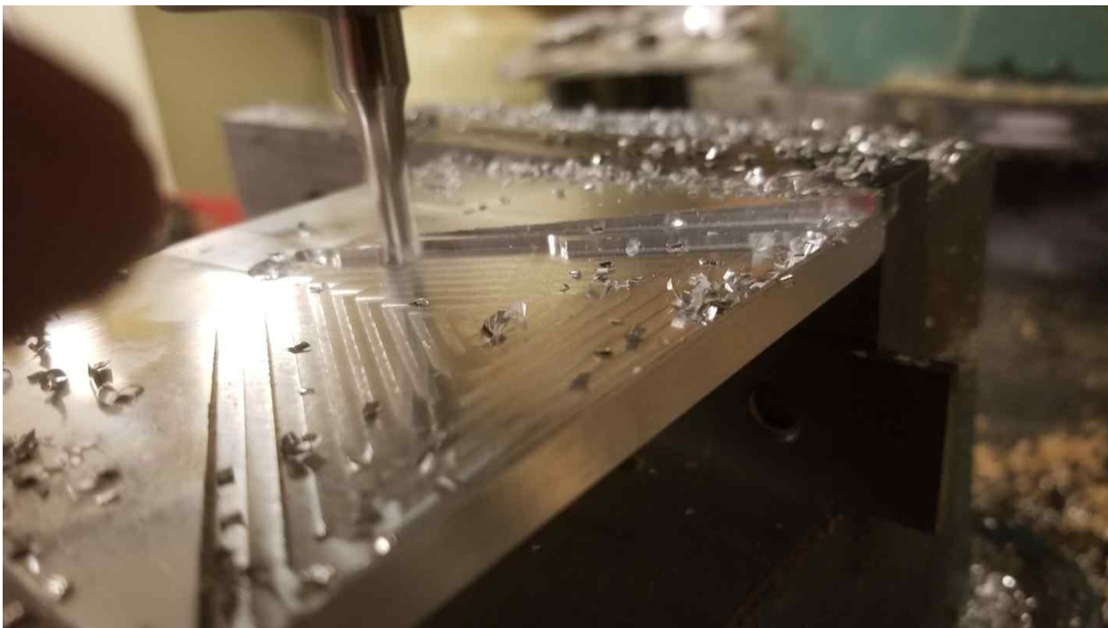
Figure 3 – Sectoral Horn half for 10 GHz being machined by CNC mill.
