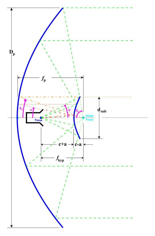
Figure 4 – Geometry of Cassegrain antenna
