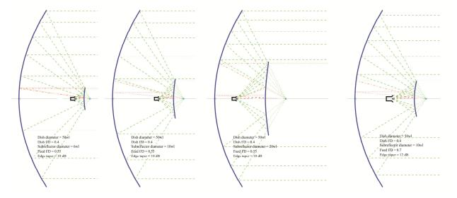
Figure 5 – Moving feed location changes size of subreflector
