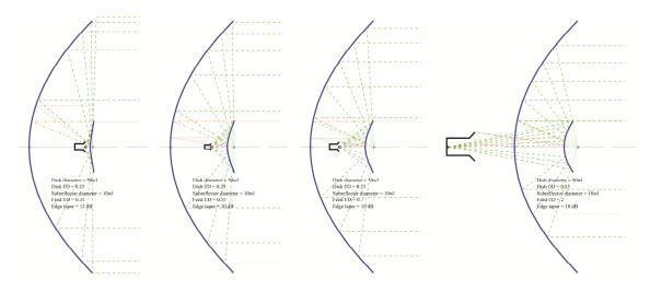
Figure 6 – Higher gain feedhorns with narrower beams are located further from subreflector
