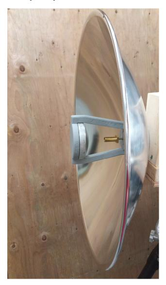
Figure 14 - 24-inch Cassegrain antenna for 47 GHz by VE2UG
