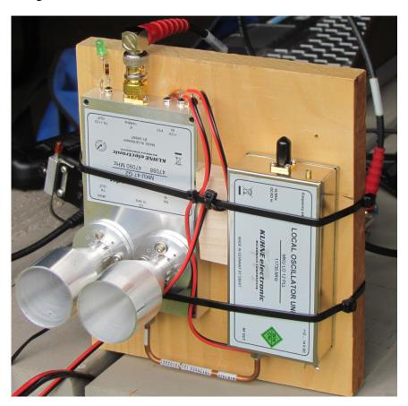
Figure 10 - DB6NT 47 GHz transverter with separate feedhorns
