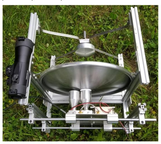
Figure 11 – Cassegrain antenna system for 47 GHz with zero feedline
