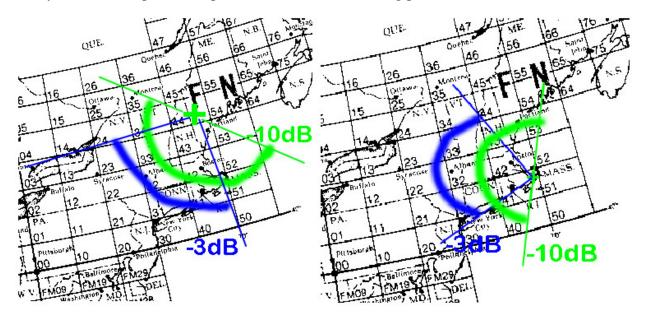
Figure 1 – An antenna pattern about 90° wide provides good coverage of New England from beacon locations in FN44, left, and FN41, right.
