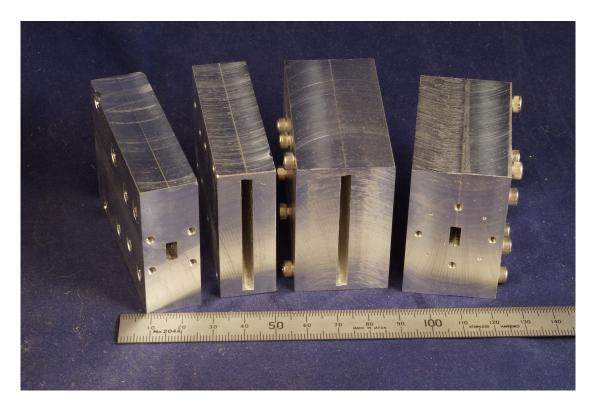
Figure 6 – Sectoral horns for 24 & 47 GHz with WR-28 waveguide input
