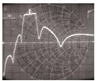
mum noise figure. If all is working well, the minimum should include a broad range of attenuation.
