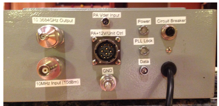
Connections on the Beacon
