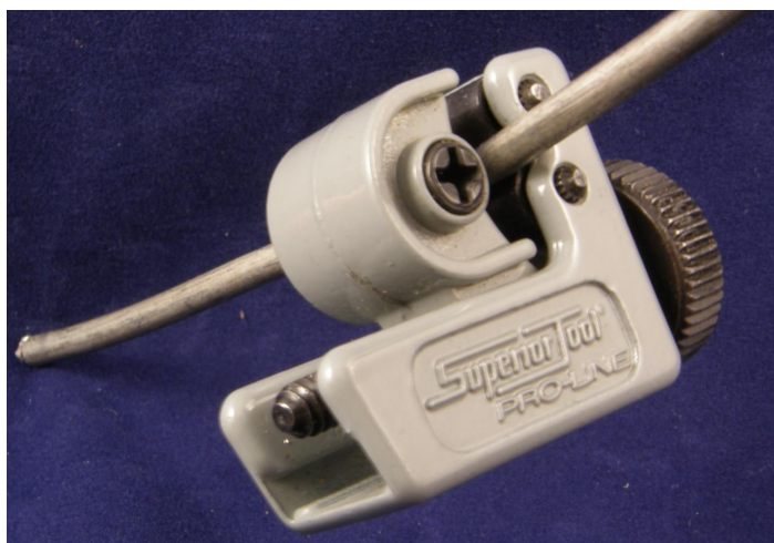
Figure 5 – Preparing semi-rigid coax with miniature tubing cutter
