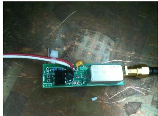
your input and output cables to the board or use connectors. I chose to put an SMA on the output to simplify testing and solder the input coax directly.
