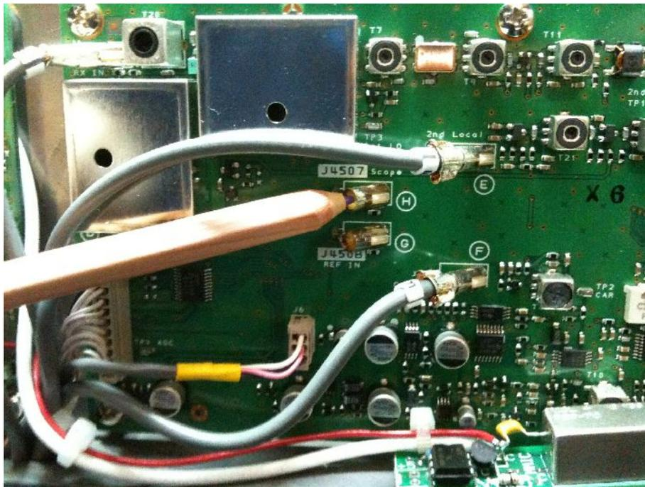
Solder up the input, drop the SMA out the back in whatever way you choice (figure 5,6), connect it up to the FunCube Dongle and follow the directions from W1GHZ and N1JEZ substituting 68.330Mhz as the IF.
