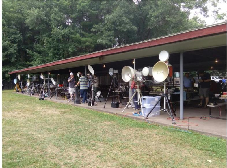
Finally, we also check relative ERP, transmitting one at a time and recording the relative power received at the distant point.
