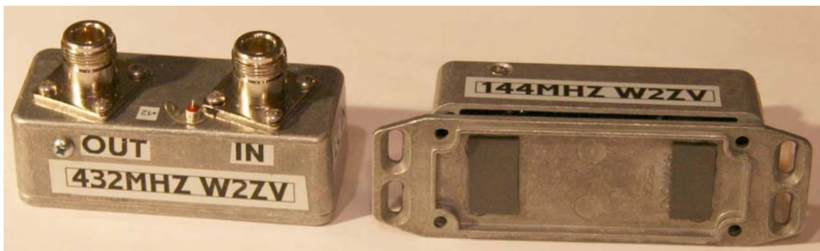
Figure 9: Finished box and cover inside with absorber applied.
