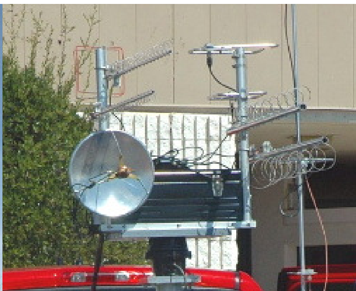
Above: The Rover "Toolbox" with all appropriate radios inside the toolbox mounted on a rotor with antennas attached.
