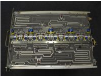
Starting point. Unmodified lo/lo 1kW amplifier.
