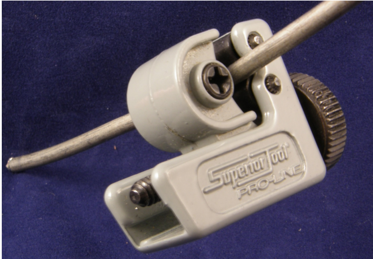
Figure 10 – Preparing semi-rigid coax with miniature tubing cutter
