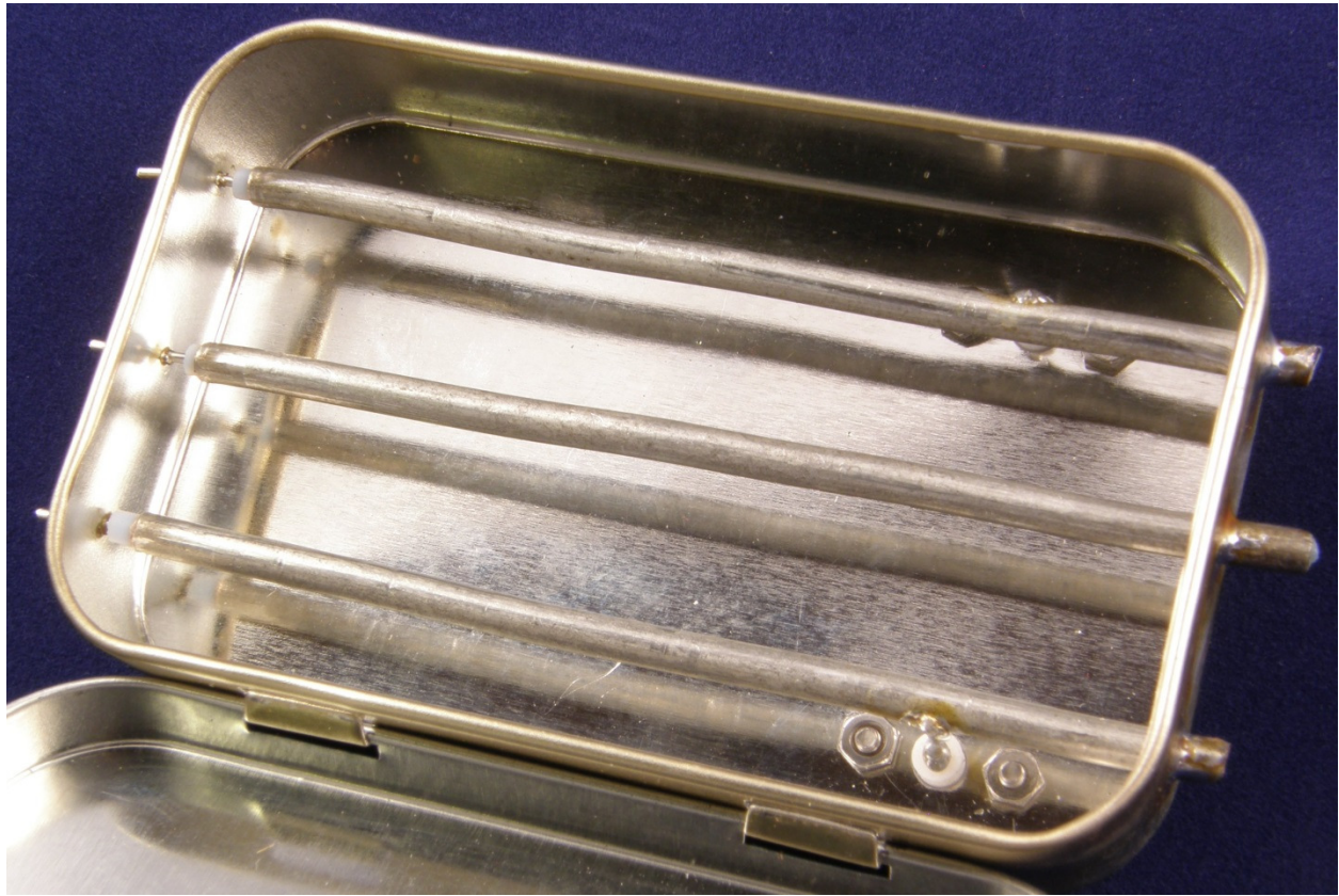
Figure 1 – 432 MHz Comblin filter in Altoids tin
