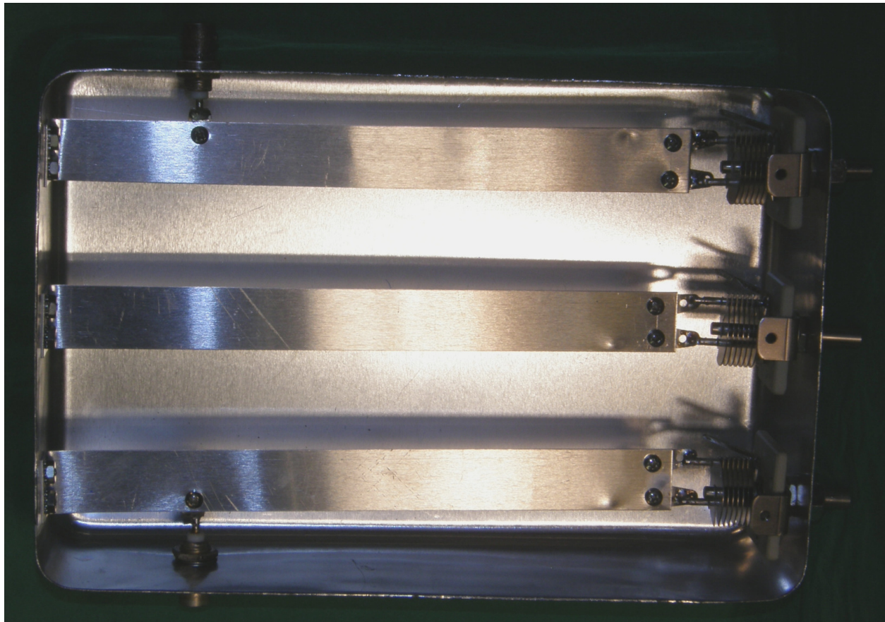
Figure 2 – Combine Filter for 144 MHz
