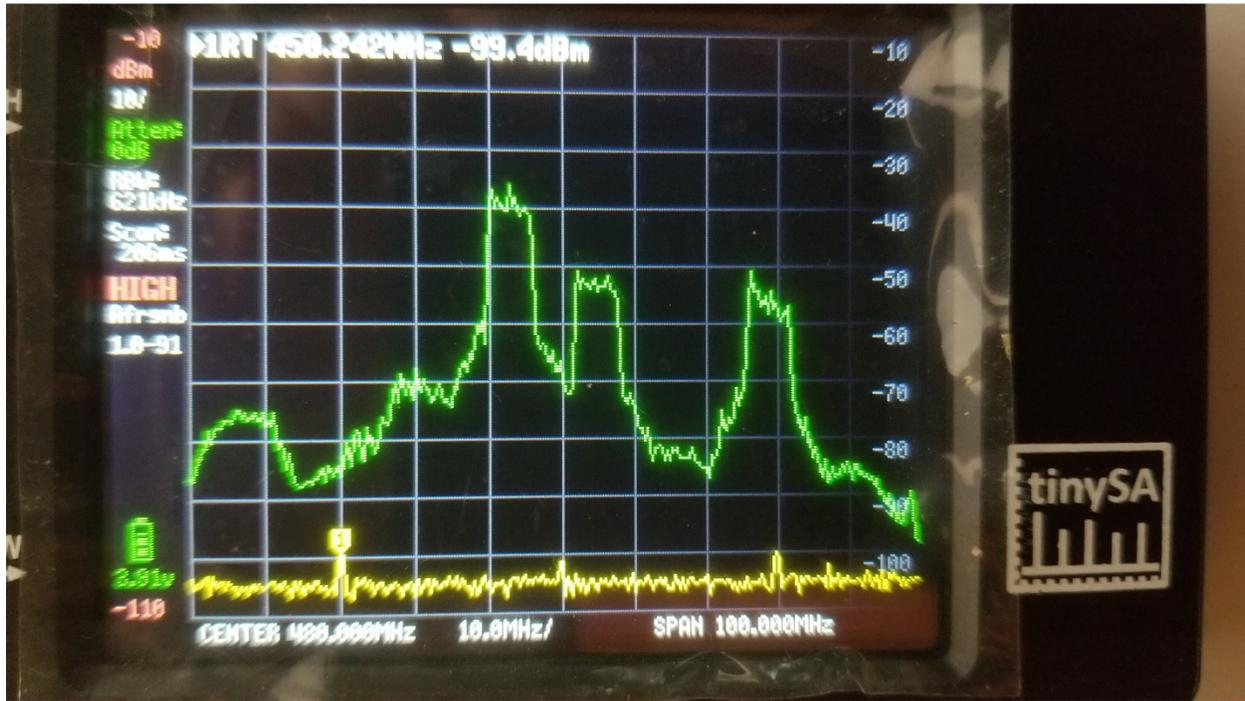
Figure 2 – DTV signals received on log-periodic antenna
