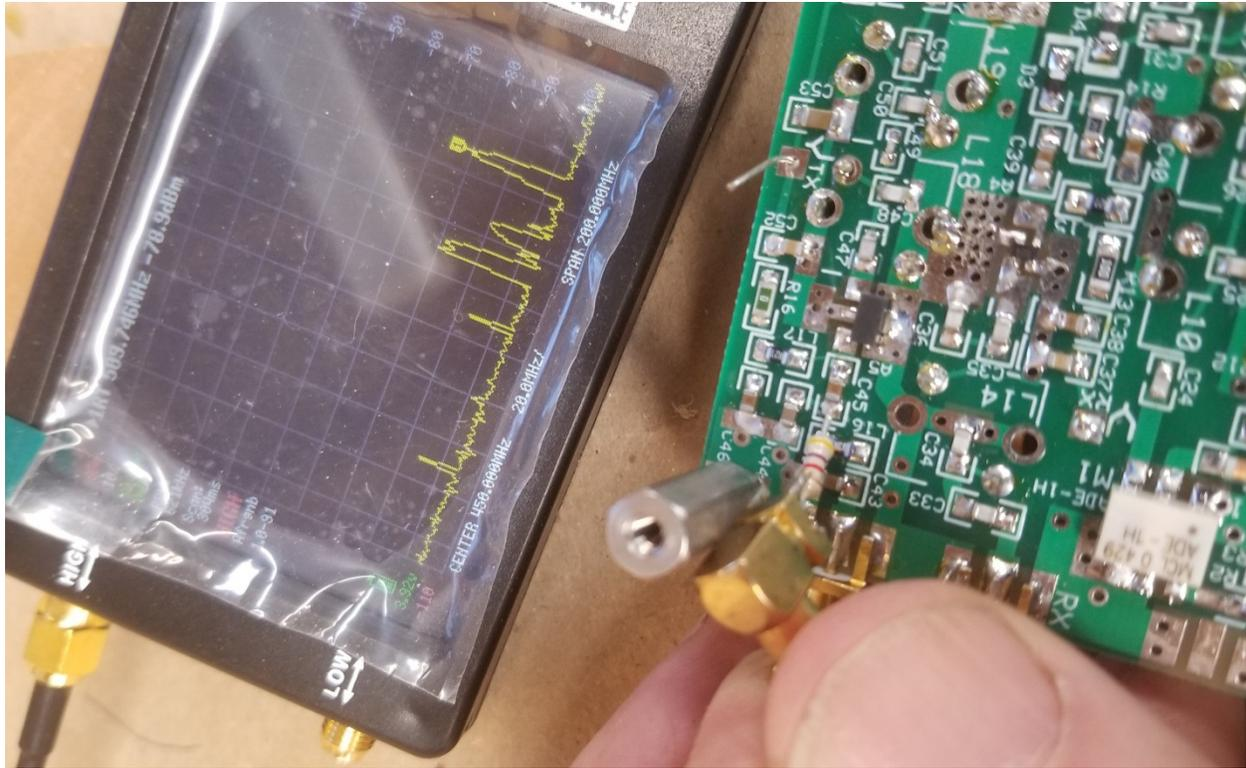
**Figure 1 – Probing RF circuit with Spectrum Analyzer thru isolating resistor**
