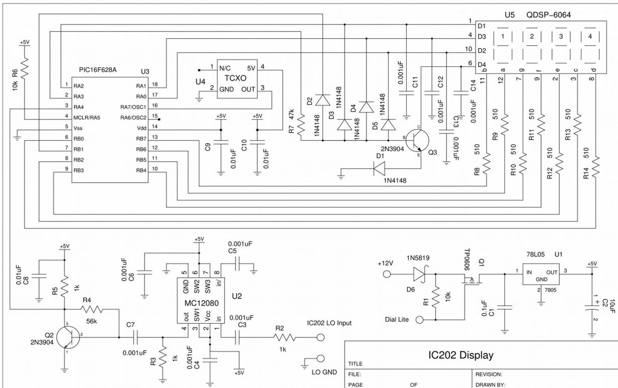
Figure 1: Display circuit
