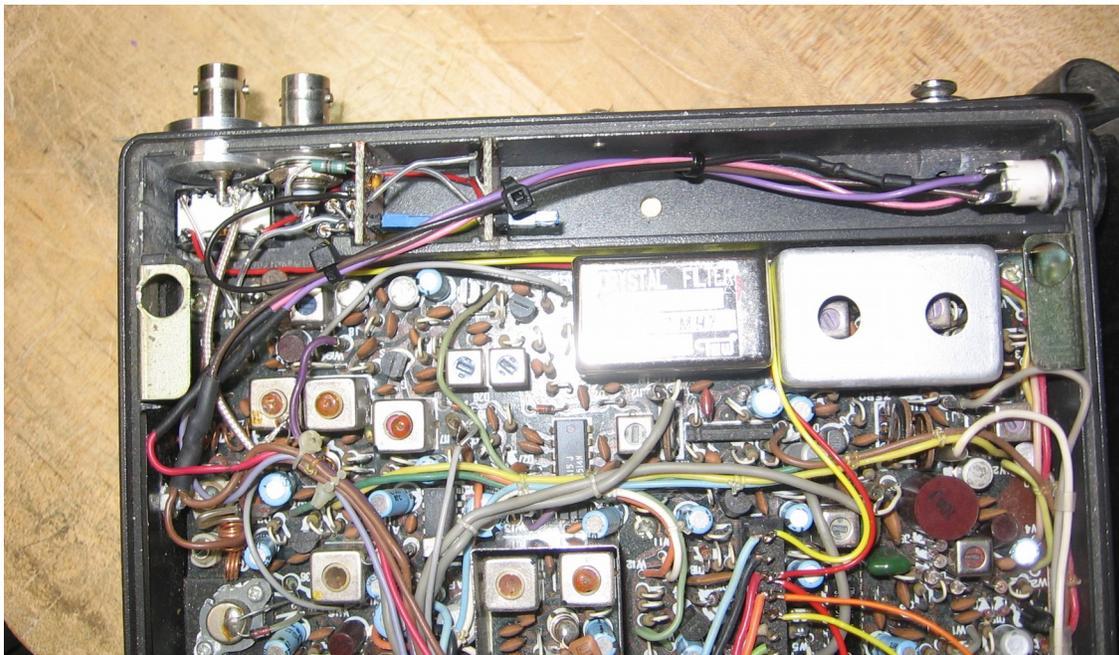
Figure 5: T/R relay and transverter circuitry. The relay is in the far upper left corner.
