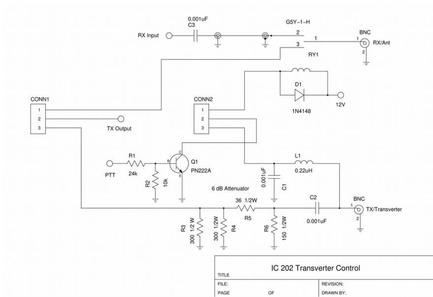
Figure 4: Transverter control circuit.
