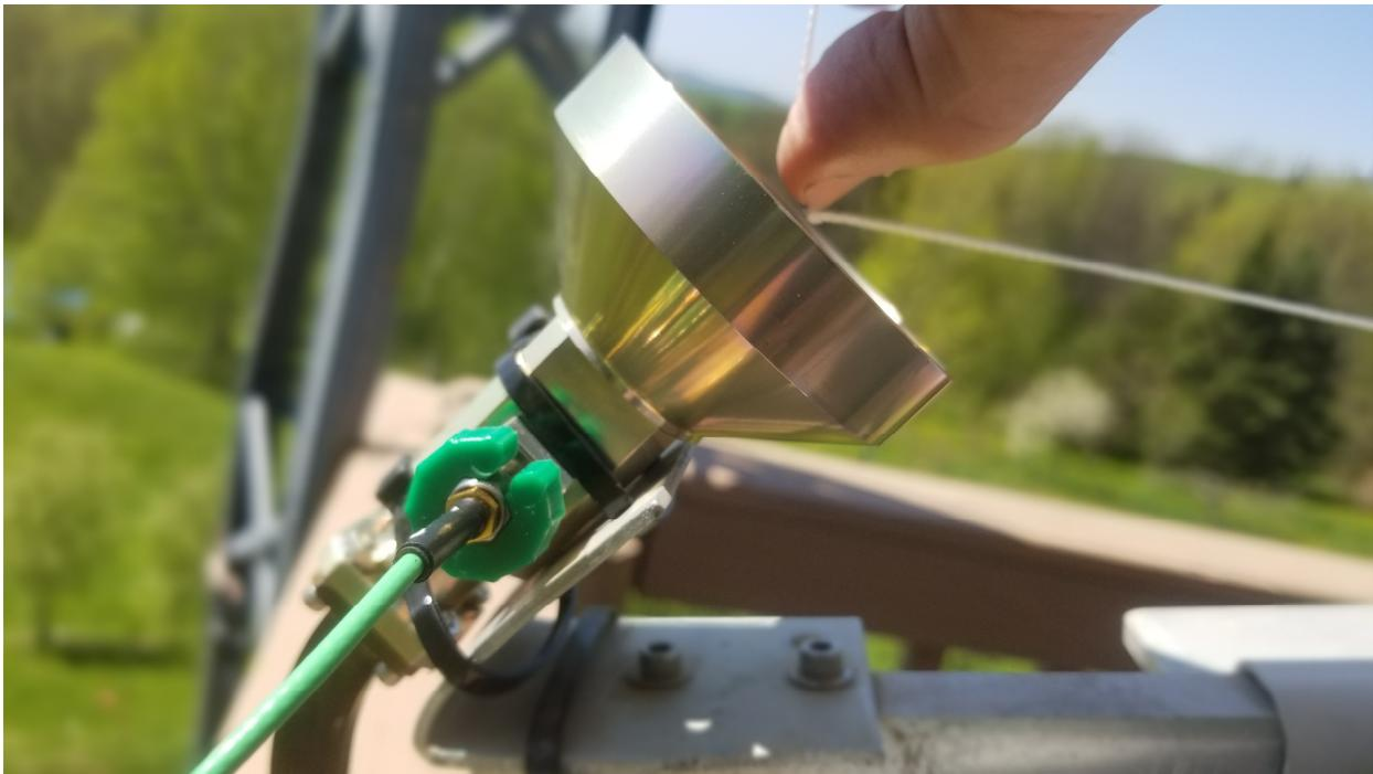
**Figure 5 – Using modified string lengths to align feed at center of aperture**
