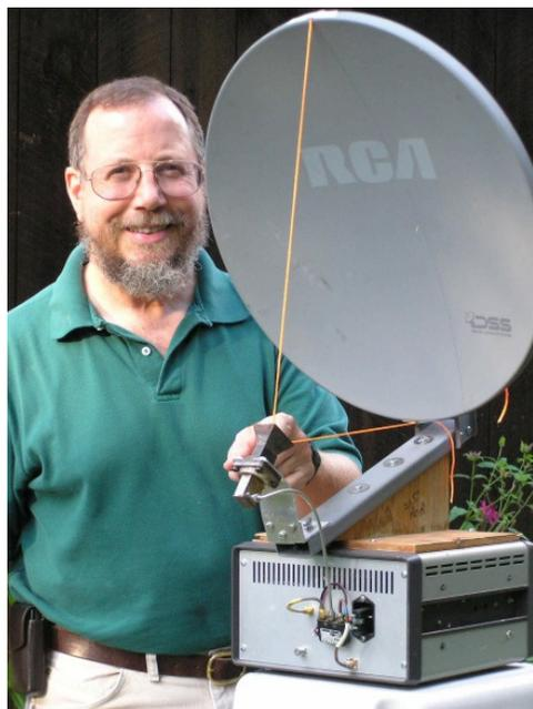
Figure 2 – Finding dish focus using string method
