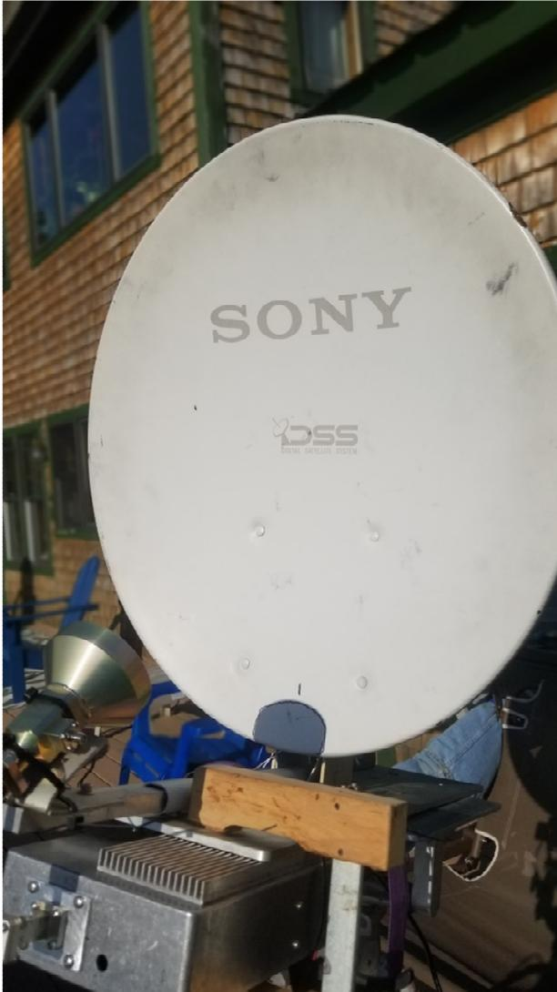
Figure 8 – Feed shadow marked on dish
