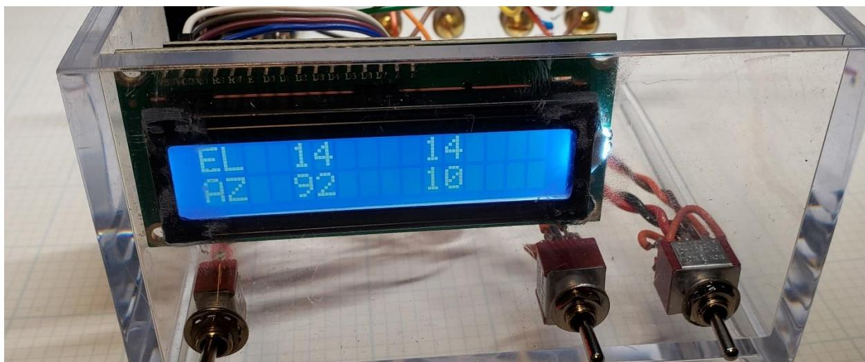
(The second column of numbers in the above display is the A-D capture of the 1024-level resolution of the wiper voltage appearing at the analog inputs of the Arduino. These numbers are handy to have during calibration of the readout as you tweak the scaling functions at the end of the program.)
