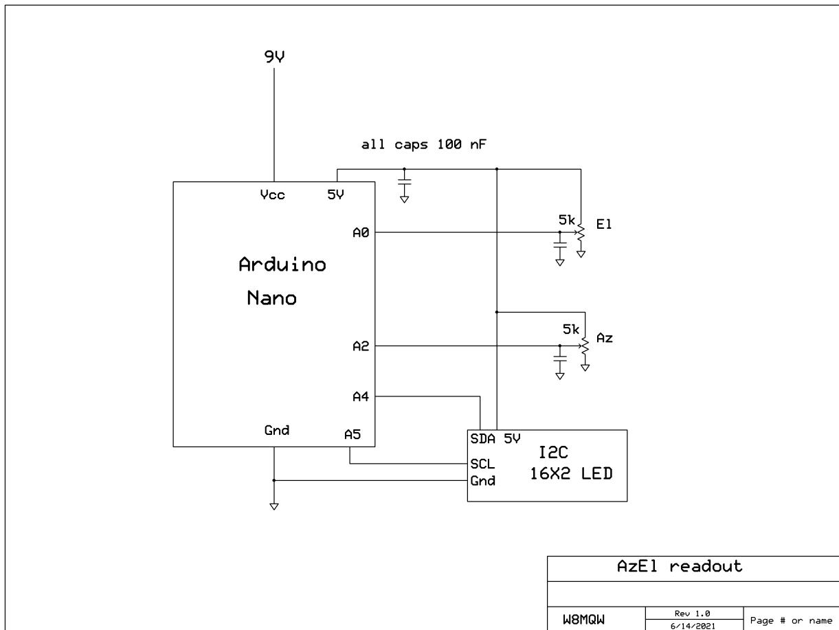
The visual display is an inexpensive 16x2 LED with a I2C daughterboard that is mounted simply with dabs of glue at its four corners into a transparent box available from [1]:
