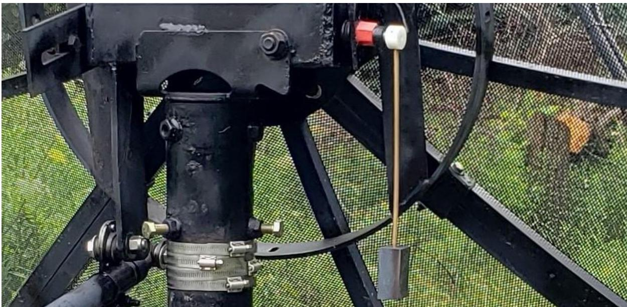
Five volts is applied to the top of each pot, the bottom grounded, and the wiper read by the Arduino in the shack. The circuit is simplicity itself:
