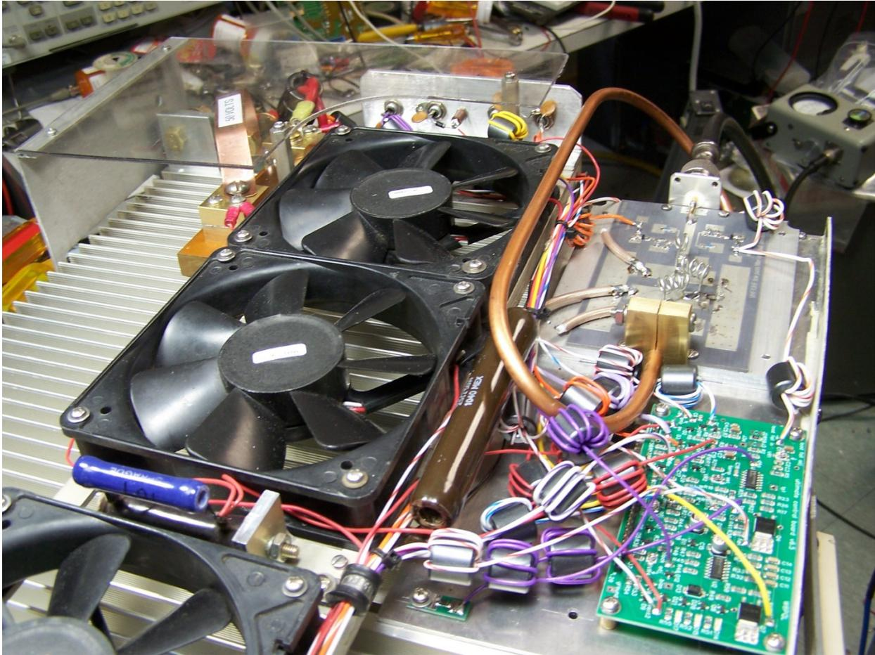
**A detailed view of the W6PQL Control Board. I wired all of the connections to the top of the board. I also used some mix 43 toroids on all of the connecting leads to control any RFI problems. For best results at 222 MHz, use no more than three turns of wire on each toroid.**
