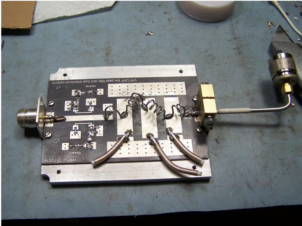
The W6PQL 222 MHz Filter modified for high power. Substrate is some ¼" aluminum plate. The chip caps have been replaced by short lengths of Teflon coax. This particular filter measured -48 dB at the 2<sup>nd</sup> harmonic, and -60 dB at the 3<sup>rd</sup> harmonic frequency. Return loss through the filter is over 30 dB.
