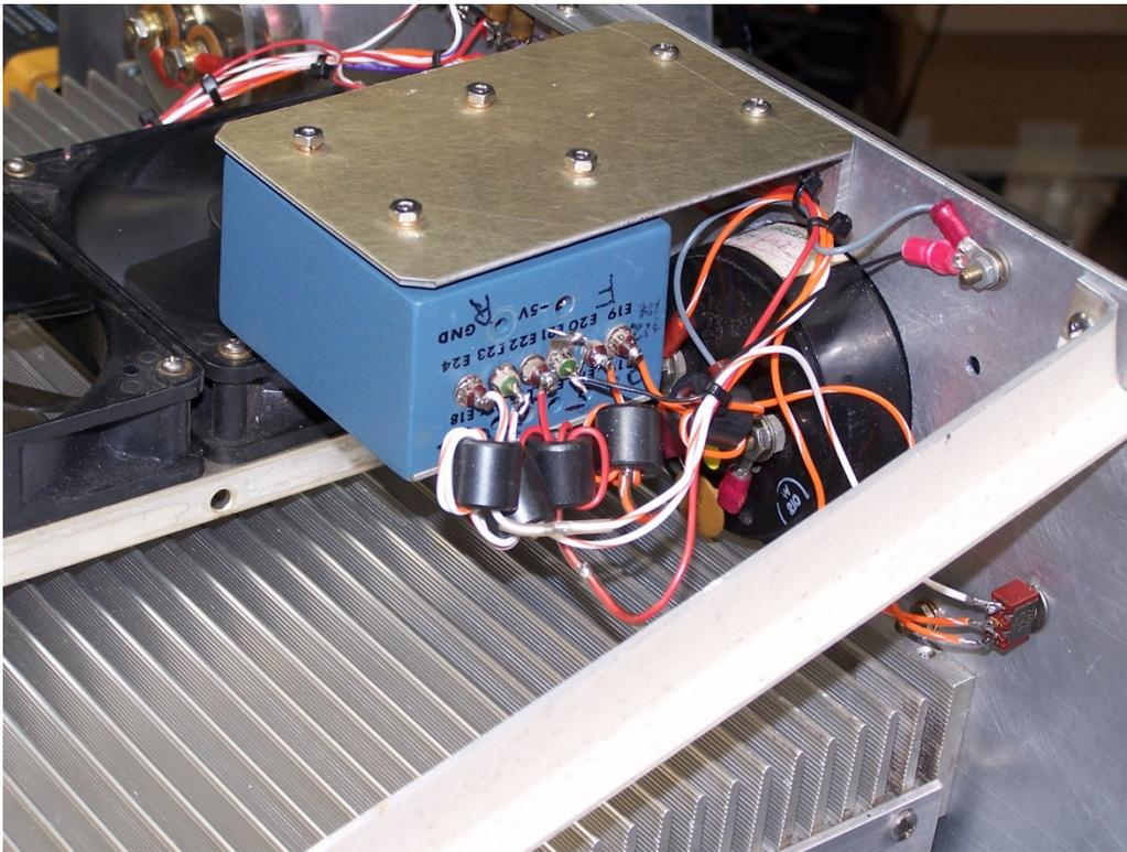
**OP-AMP METER DRIVER BOARD in an RF proof enclosure is mounted on the front panel near the power meter. There are two multi turn potentiometers inside the enclosure that adjust forward and reflected power through two access holes. Note the front panel side brace.**
