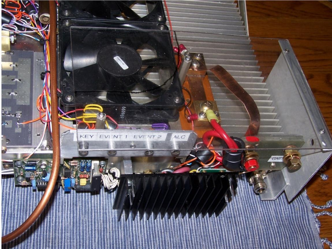
**Here is the right rear portion of the amplifier. The Larcan protection board is on the left. The black heat sink in the middle contains the FET DC switch. The 50 volt power terminals are on the far right.**
