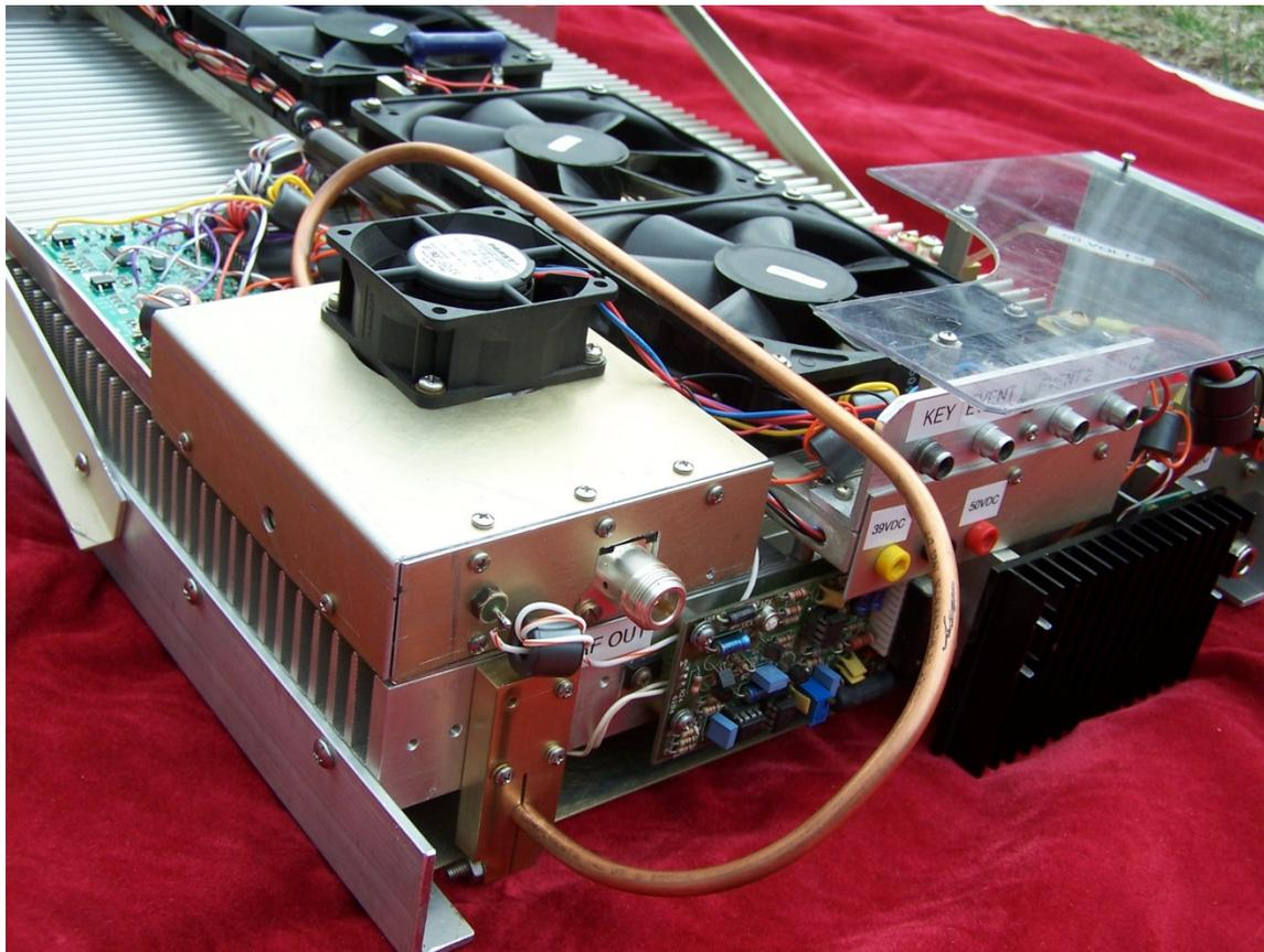
**This is the final version of the amplifier with a metal enclosure over the output filter. Note the cooling fan to keep the filter components cool. It is a small 24 VDC fan with a 500 ohm dropping resistor from the 50 volt buss to limit noise but still provide adequate cooling for the filter coils.**
