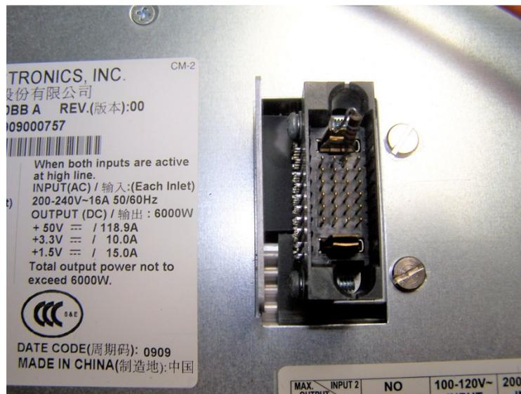
**Cisco DPST 6000BB Power Supply. “ENABLE” connections to activate the 50 volt output. Connect 3<sup>rd</sup> pin from left on top right (as shown) to the adjacent large blade connector pin with a 500 to 1K resistor.**
