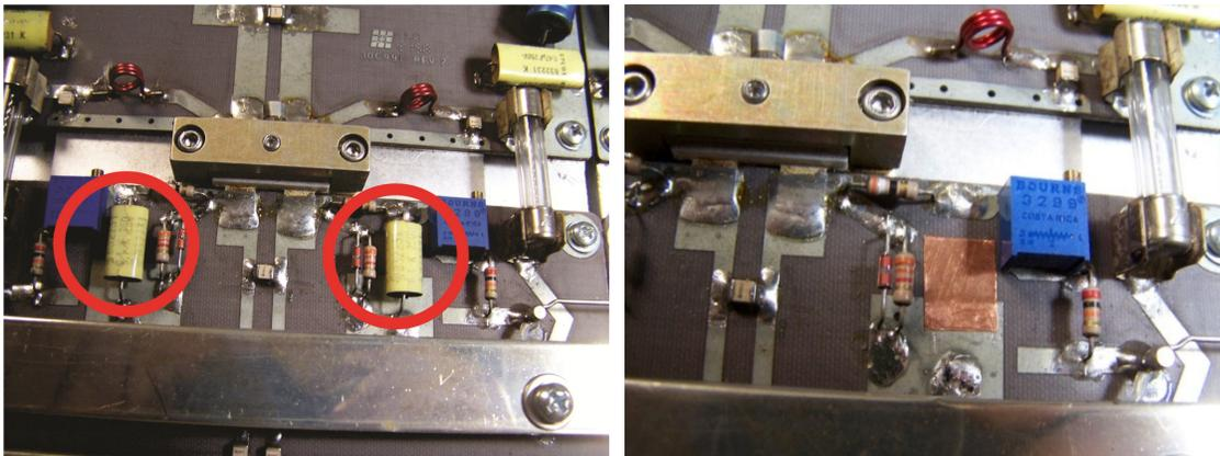
**A View of the bias circuit of the four FET 222 MHz Larcan amplifier. The yellow polyester cap on the left photo is the only bias bypass capacitor and it has rather long leads especially for 222 MHz. The 0.50" X 0.35" copper foil addition can be seen in the right photo all ready to accept the two chip cap bypass caps. NOTE THAT THESE CHANGES ARE NOT NEEDED IN THE LARGER SIX FET AMPLIFIERS.**
