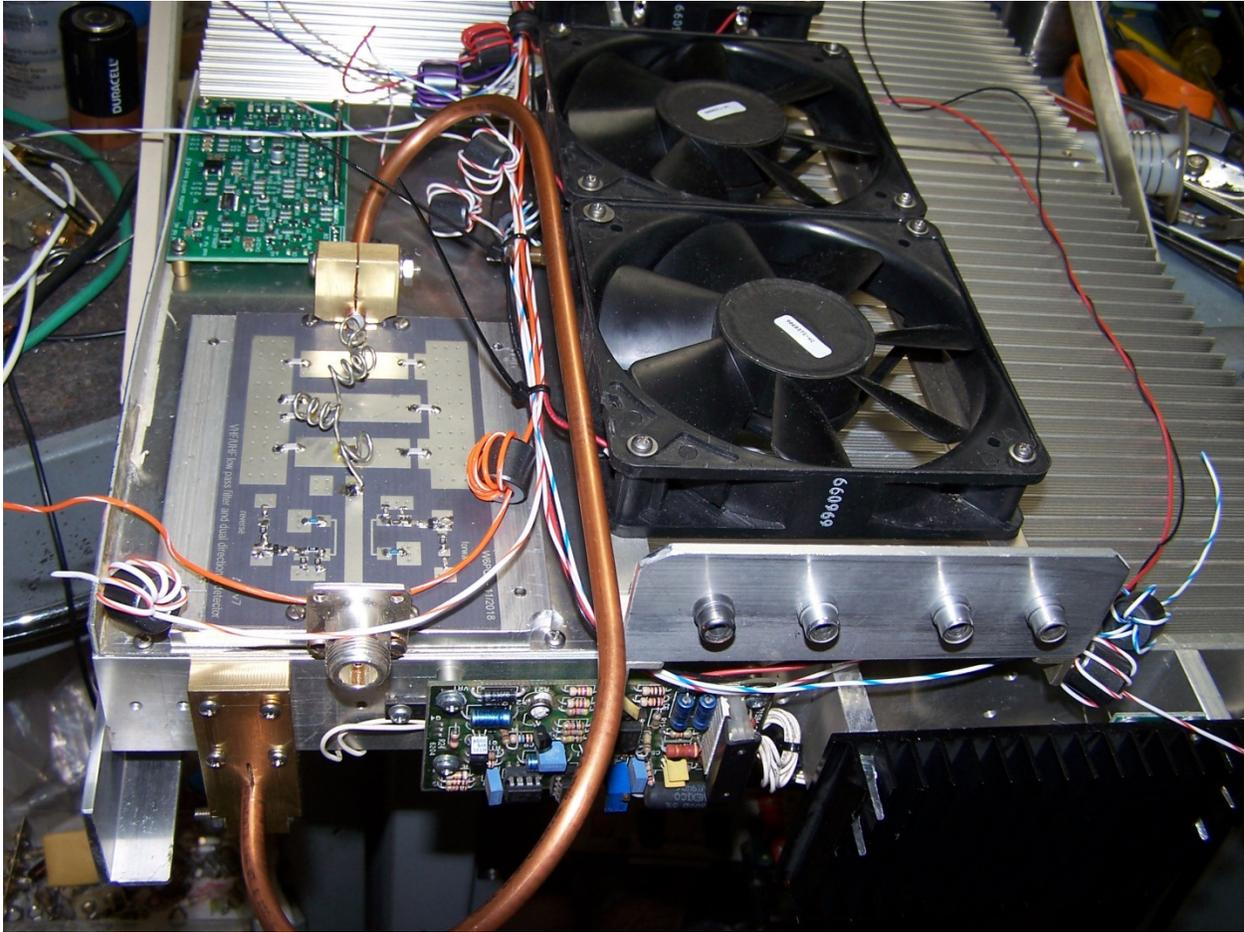
**This is a photo of the back of the amplifier while under construction. The RF filter board sits on top of the main heat sink. The W6PQL Control Board is seen in the back ground just behind the RF filter.**
