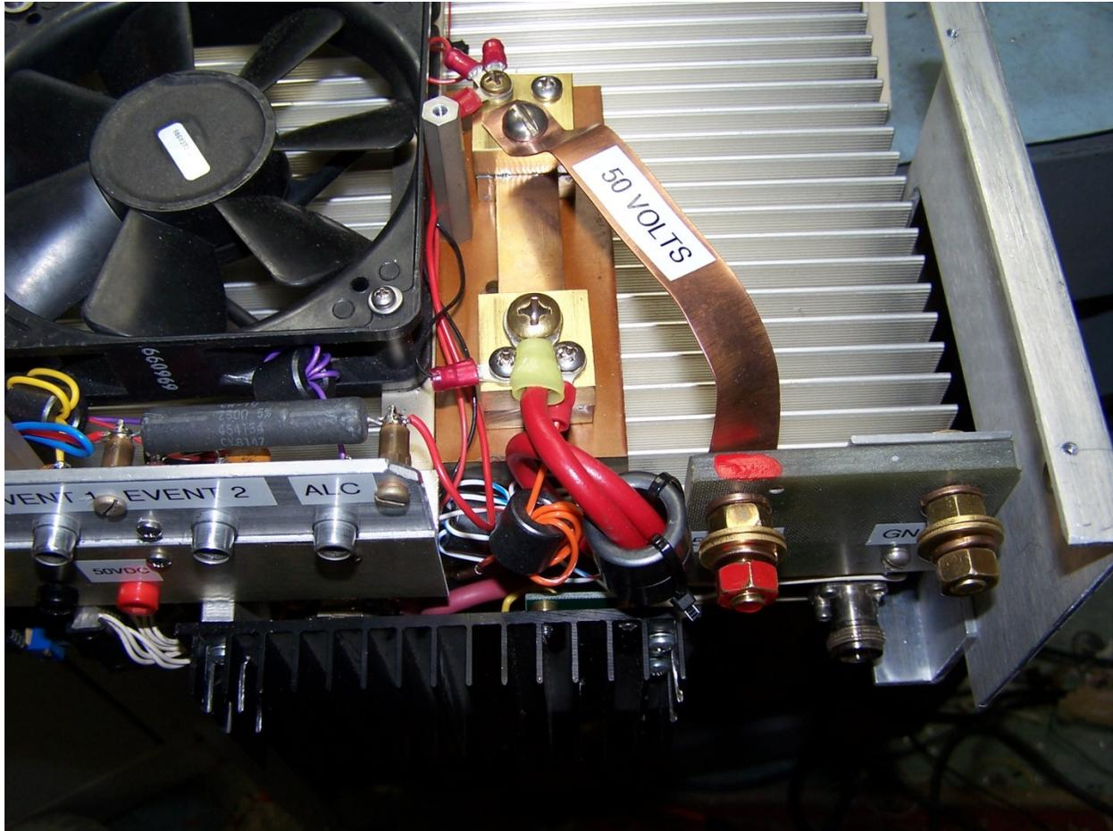
**Close up view of the home brew 100 amp shunt and the fiberglass DC input panel. I used 5/16" brass hardware. The negative terminal is directly grounded to part of the aluminum chassis, while the positive lead runs over to the shunt. The big red wire and ferrite donuts attach to the FET DC switch mounted on the black heat sink that extends behind the main chassis/ heat sink.**
