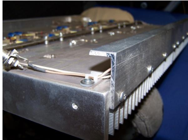
**Aluminum channel stock is used for the side rails. Size is  $\frac{3}{4}$  X 1  $\frac{1}{2}$  X 1/8" wall. (This picture is of a 4 FET amp)**
