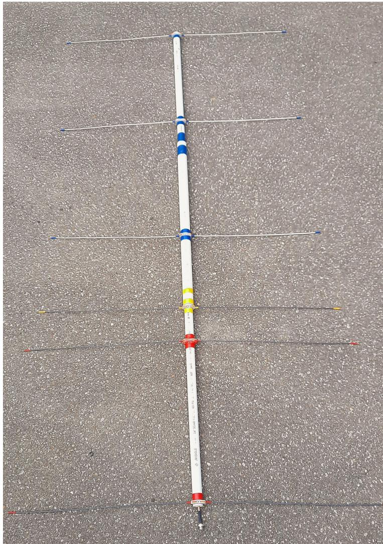
The connectors are not waterproof so this is not an all-weather antenna. The +/- connection at the feed is particularly sensitive to water. The impedance may change when wet. {Would those then be rain scattering parameters?}
