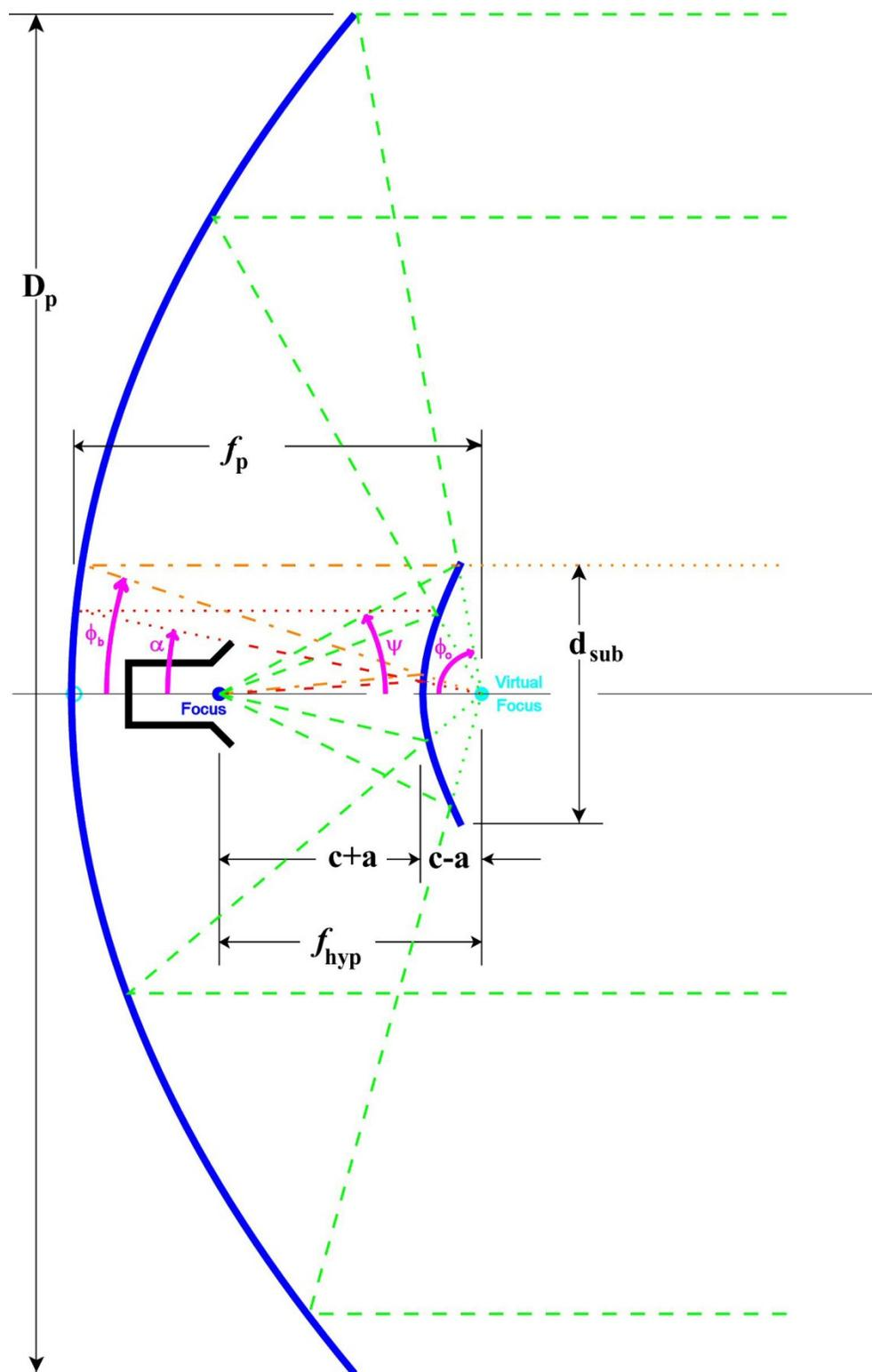
Figure 4 – Geometry of Cassegrain antenna
