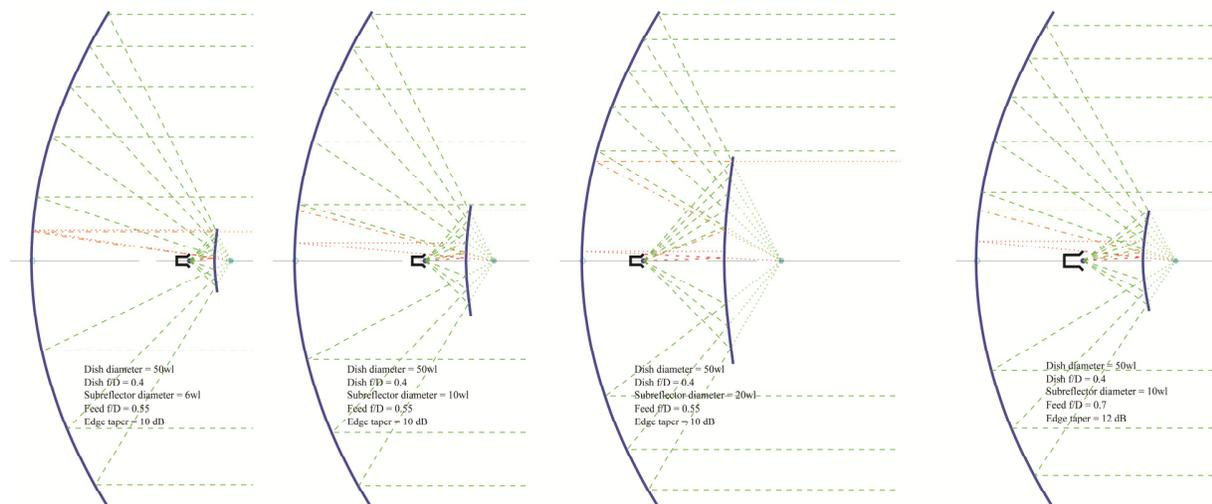
**Figure 5 – Moving feed location changes size of subreflector**
