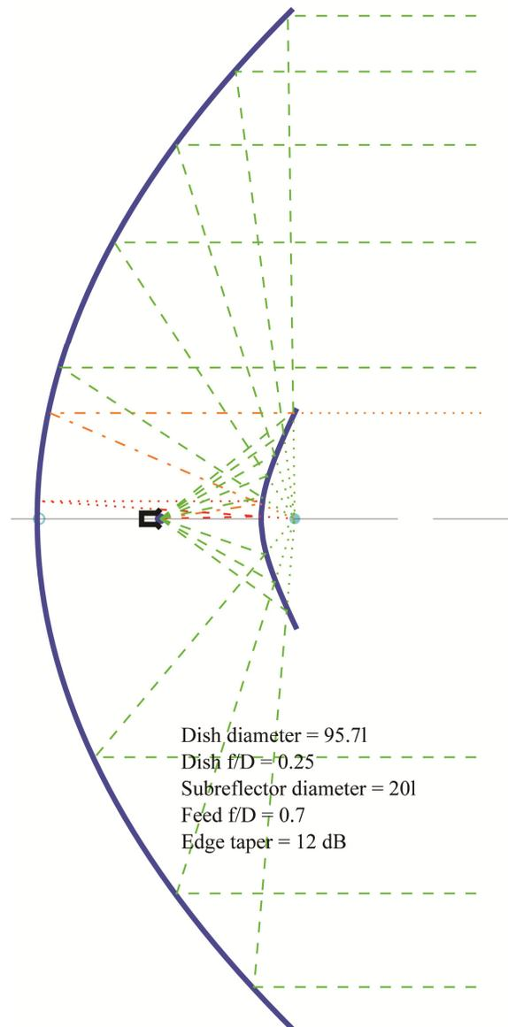
**Figure 13 - Cassegrain antenna for 47 GHz with 609mm dish,  $f/D = 0.25$**
