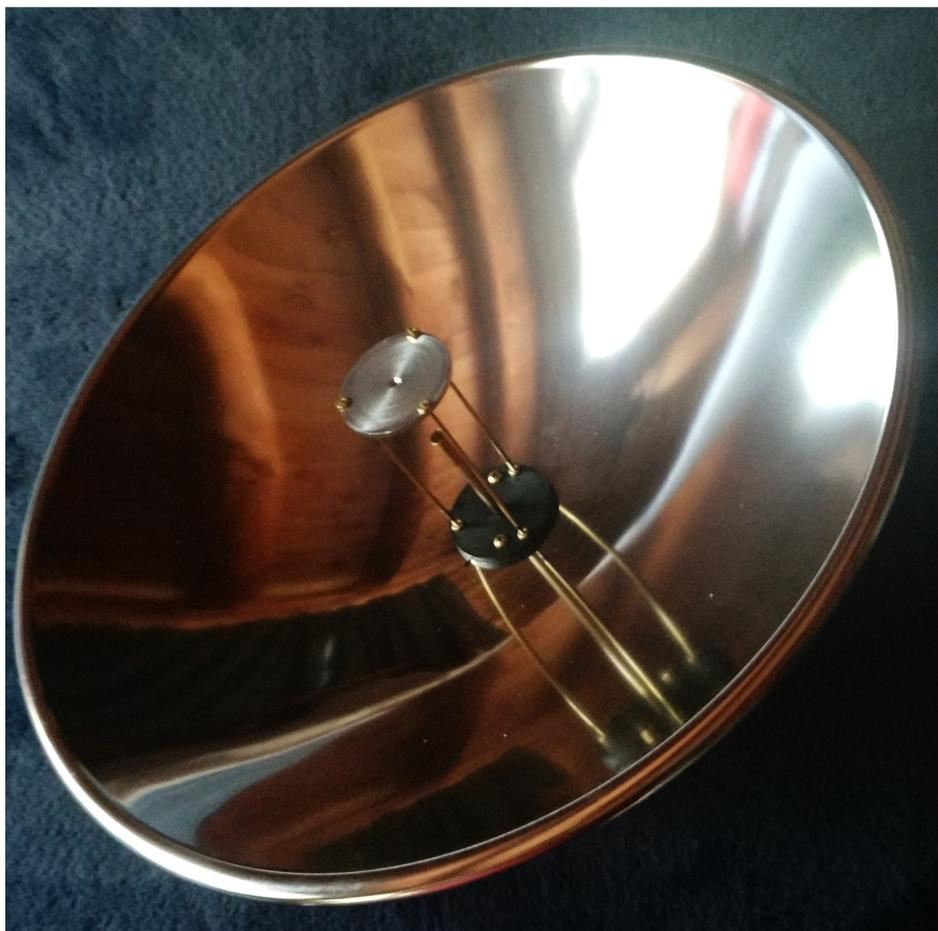
**Figure 8 - Cassegrain antenna for 122 GHz with 305mm dish by W1FKF**
