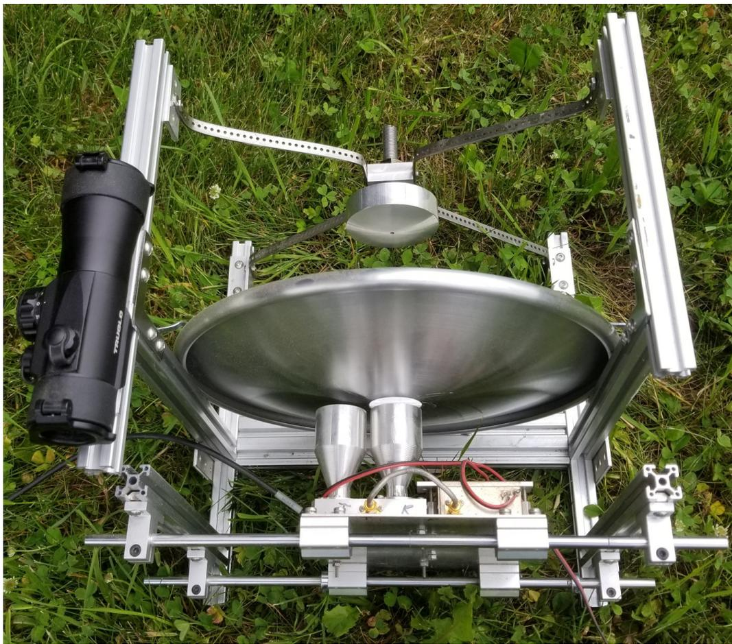
**Figure 11 – Cassegrain antenna system for 47 GHz with zero feedline**
