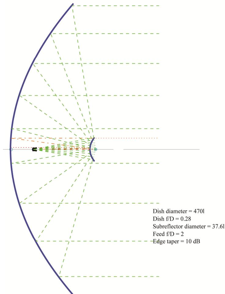
**Figure 15 - Cassegrain antenna for 24 or 47 GHz with 3m dish,  $f/D = 0.29$**
