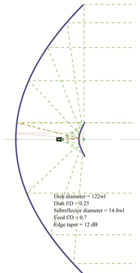
**Figure 7 – Cassegrain antenna for 122 GHz with 305mm dish,  $f/D = 0.25$**
