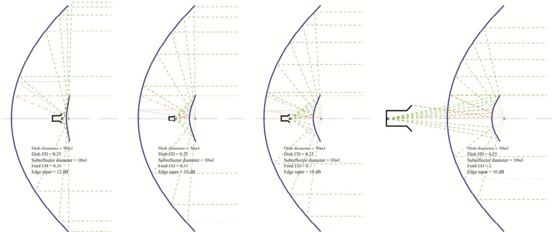
**Figure 6 – Higher gain feedhorns with narrower beams are located further from subreflector**
