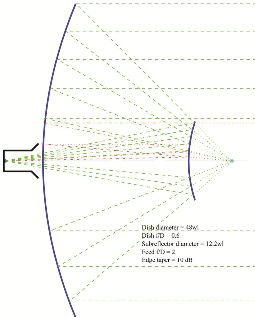
Figure 9 - Cassegrain antenna for 47 GHz with 305mm dish,  $f/D = 0.6$
