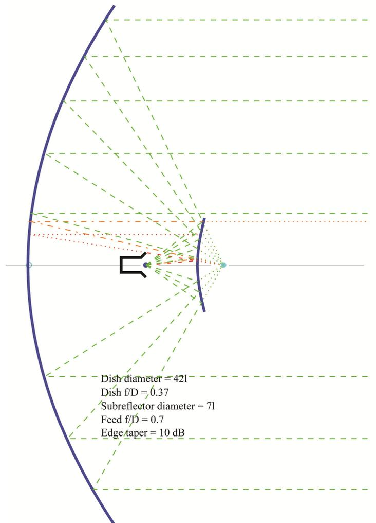
Figure 12 - Cassegrain antenna for 10 GHz EME with 1.2m dish,  $f/D = 0.375$
