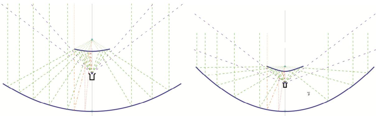
**Figure 1 – Spillover from feedhorn is directed at cold sky**
