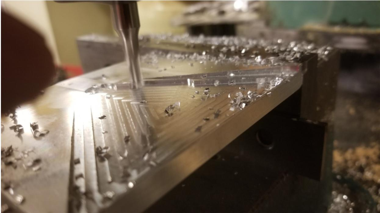
**Figure 3 – Sectoral Horn half for 10 GHz being machined by CNC mill.**
