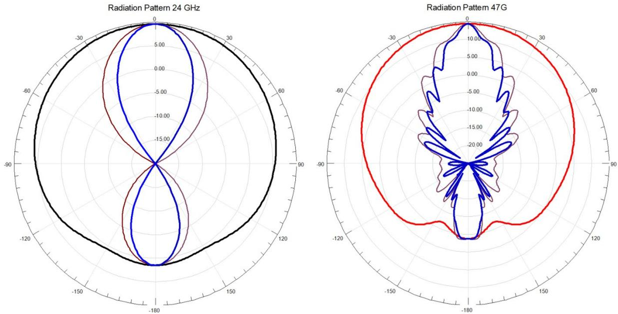
**Figure 5 – Radiation patterns for WR-28 sectoral horn at 24 GHz and 47 GHz**
