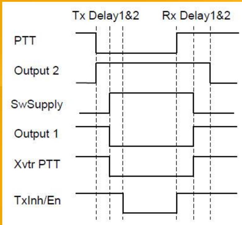
TxInh/En when hi inhibits RF
