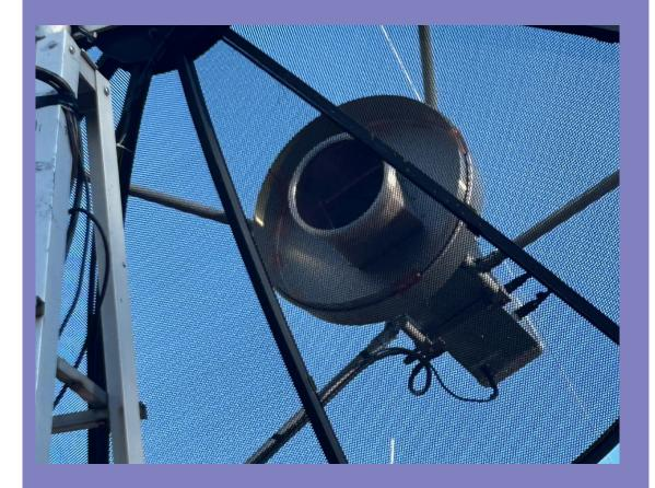
OK1DFC Septum Feed Feed Fiberglass Struts Preamp WD5AGO .3 dB nf 35 DB gain preamp Isolation Rx Relay In Back section of Feed
