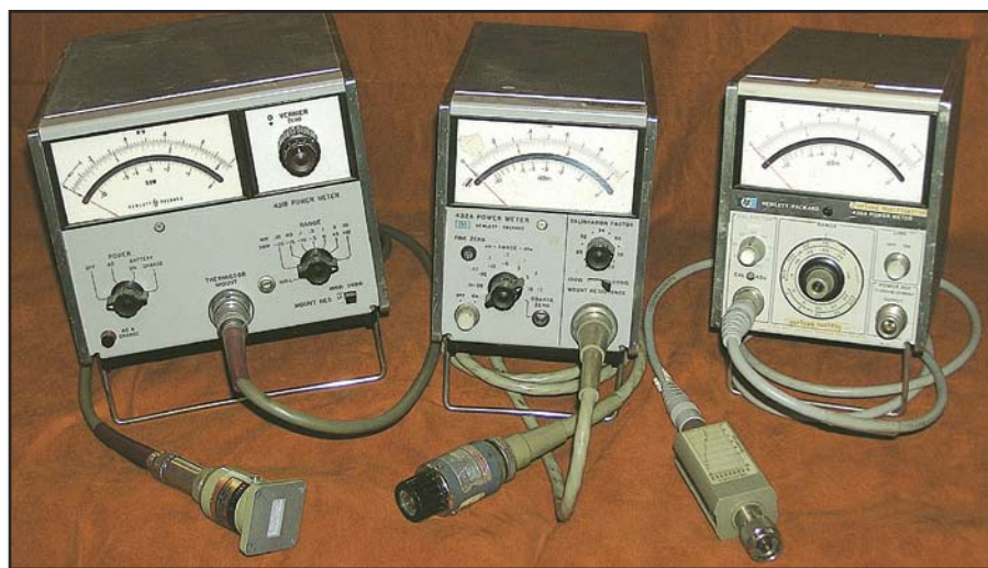
The HP models 431, 432 and 435, surplus microwave power meters with waveguide and coax sensors.
