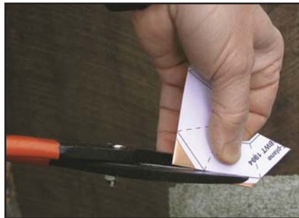
Figure 4—Using the template to cut out the horn.
