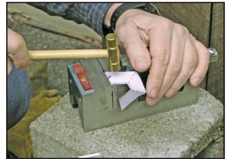
Figure 5—Bending the horn along the fold lines.
