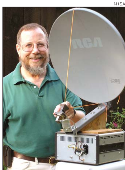
Figure 4—To locate the feed, I tie a knot in some string, then tape the string to the edges of the dish so the knot is the required distances from the edges.
