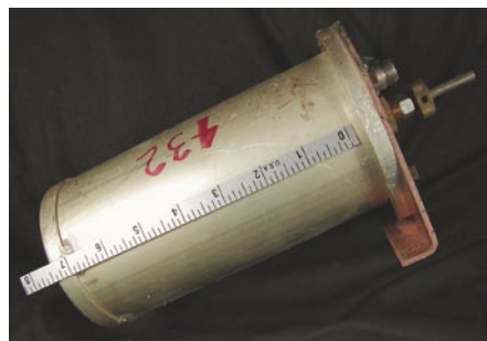
Figure 1 — Cavity filter for 432 MHz.
