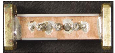
Figure 5 — External view of a 24 GHz waveguide filter made by W2PED.
