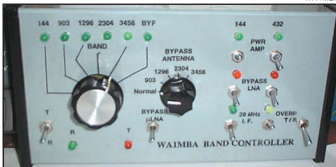
Figure 5—Here is a photo of a home built microwave band switch and sequencer. Many possibilities for control result in different designs, including indicating lights and override or bypass control.
