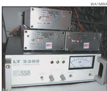
Figure 1—Here is a stack of transverters in a home station. The top ones from Down East Microwave are for 903, 2304 and 3456 MHz, and the bottom one from SSB Electronic is for 1296 MHz. Other homebrew transverters for 5760 and 10,368 GHz are elsewhere in the shack.
