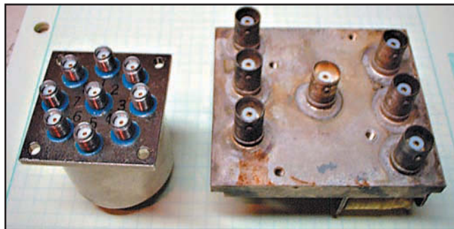
Figure 4—Two examples of multiport coaxial relays suitable for routing IF signals between one IF rig and multiple transverters. On the left is an 8-port SMA type. On the right is a 6-port BNC type.
