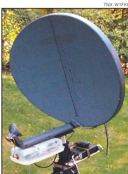
Figure 4—A string on the front of the dish will cast a shadow onto the line on the dish when pointed at the same azimuth as the sun.
