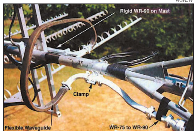
Figure 3—For those who want the minimum loss, flexible waveguide might be the answer.
