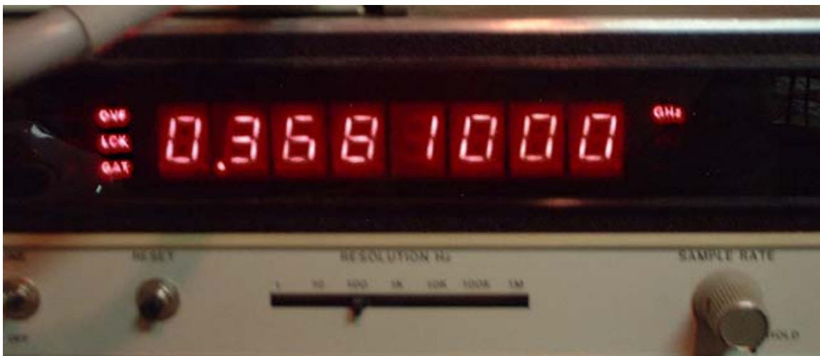
Figure 1. Here is a nice readout (there is a “1” off scale to the left) showing a 10 GHz CW signal “on frequency” to 100Hz – if the time-base standard for the frequency counter is accurate!
