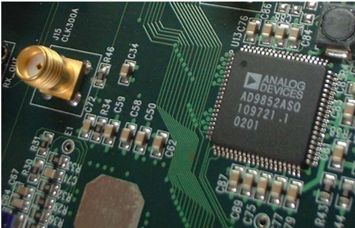
Figure 5. Here is a close-up photo of a surface mount version of the AD9852 used for the accompanying plots.
