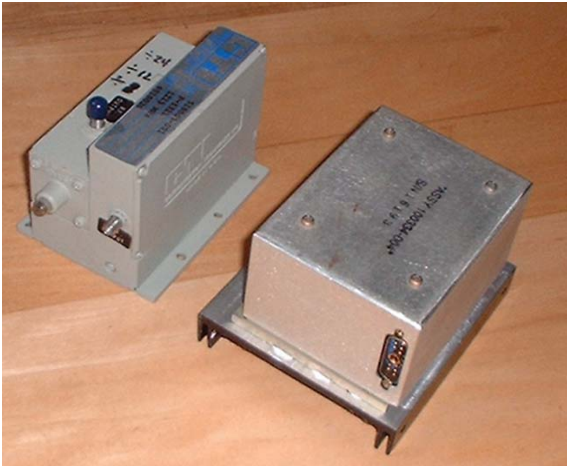
Figure 2. This photo shows a rubidium standard on the right, and for size comparison a “brick” oscillator on the left.
