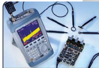
R&S®FSH with near-field probe set and DUT
