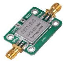
This RF Amplifier features low noise figure, is a LNA RF Amplifier.
