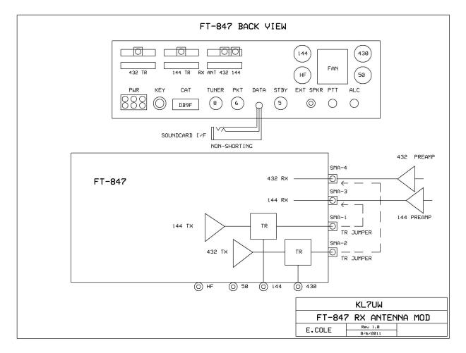
I used square flange mounting SMA connectors for my radio and soldered the RG-174 coax to the base of the pcb coax connectors and did not use the jumpers. The SMA connectors were mounted to the vent openings on the rear of the radio. This required drilling only two small holes for the 2-56 mounting screws.
