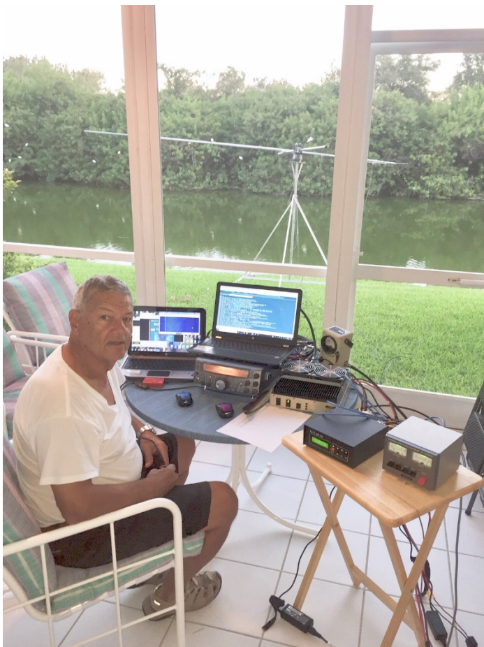
Here's the minitower in place with a single Yagi for EME.
