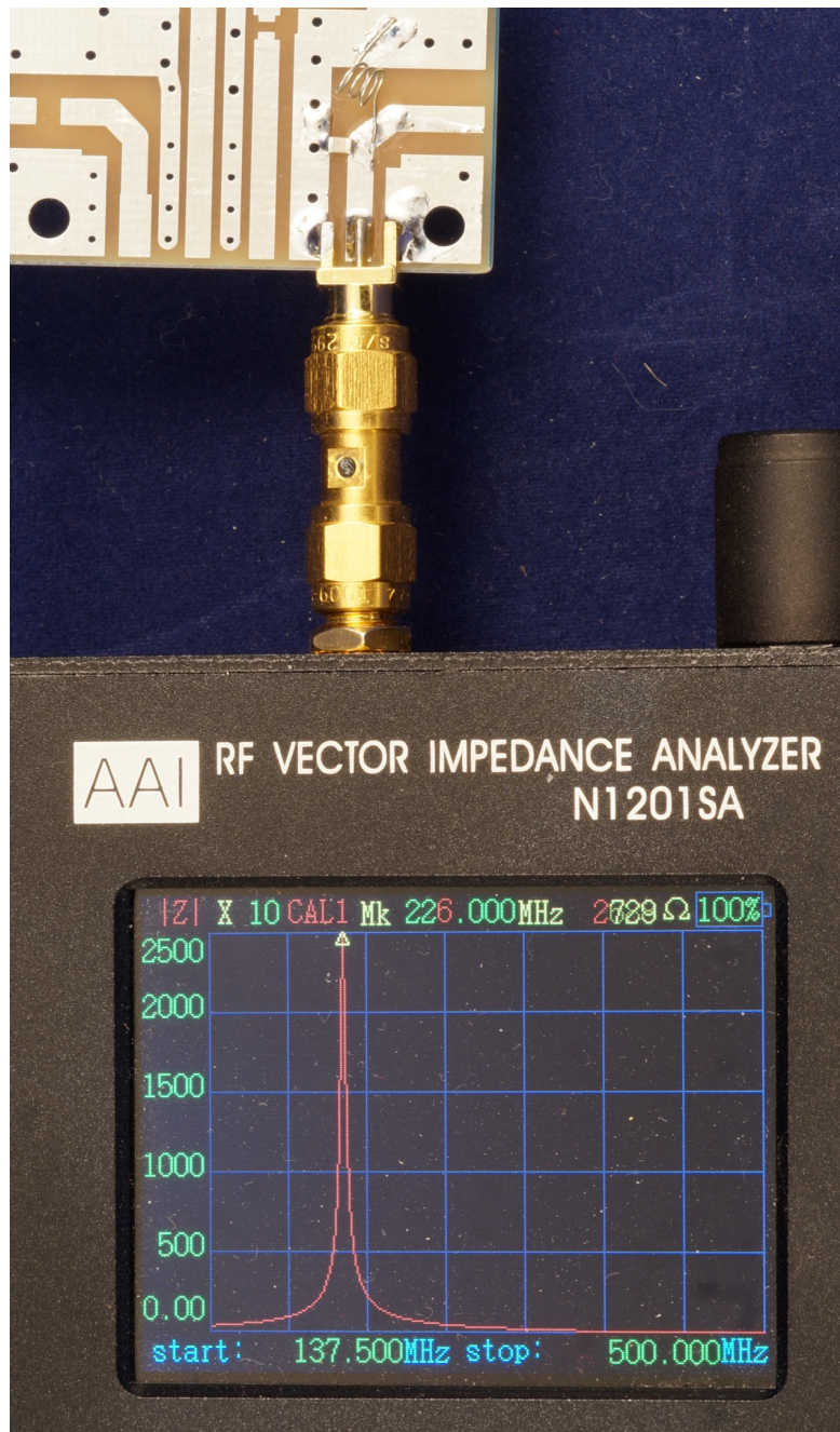
Figure 11- Measuring resonant frequency of L-C circuit with Antenna Analyzer to find inductance
