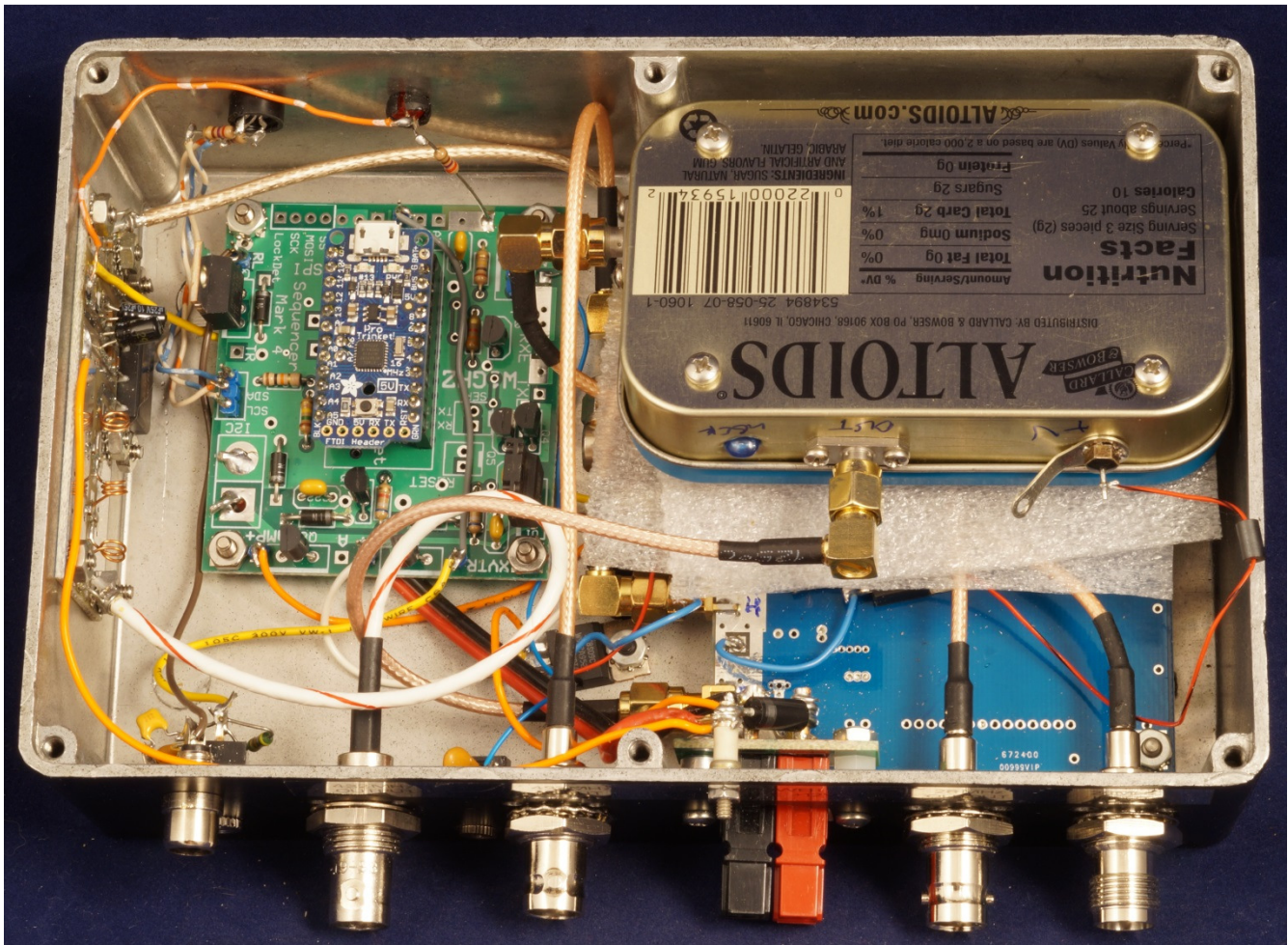
Figure 15 – Complete transverter in box with LO in Altoids tin, which attaches to cover
