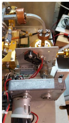
Figure 6 Motorized waveguide relay
