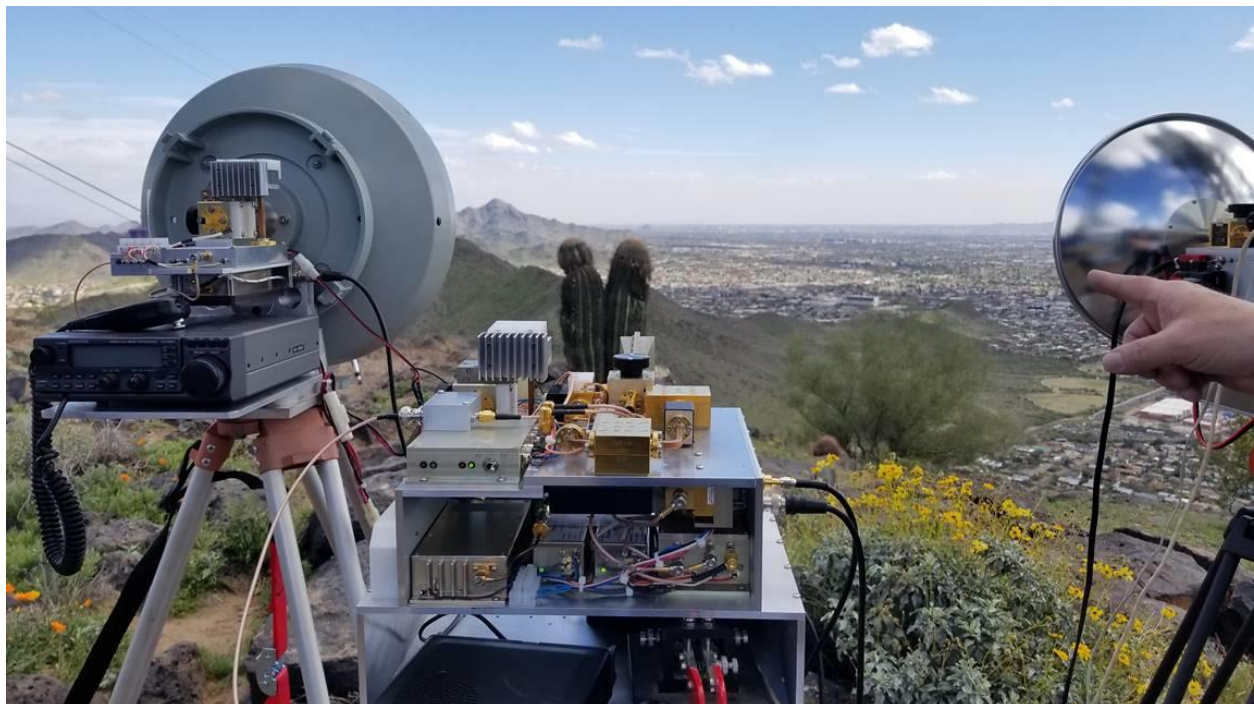
L. to R.: N0IO 47 GHz, N0IO 78 GHz with horn antenna and N0IO 78 GHz. Photo: AD7OI.
