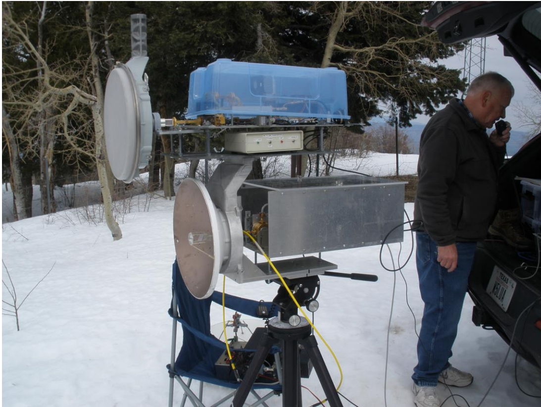
W5LUA: 47 GHz (upper) and 78 GHz. Photo: K8ZR.
