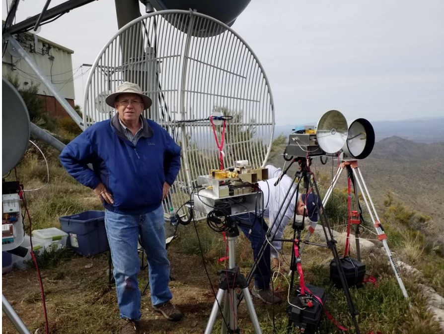
Bill W7QQ with N0IO's backup 78 GHz system with horn antennas. Bill easily worked VE4MA & W5LUA @ 207km Photo: AD7OI
