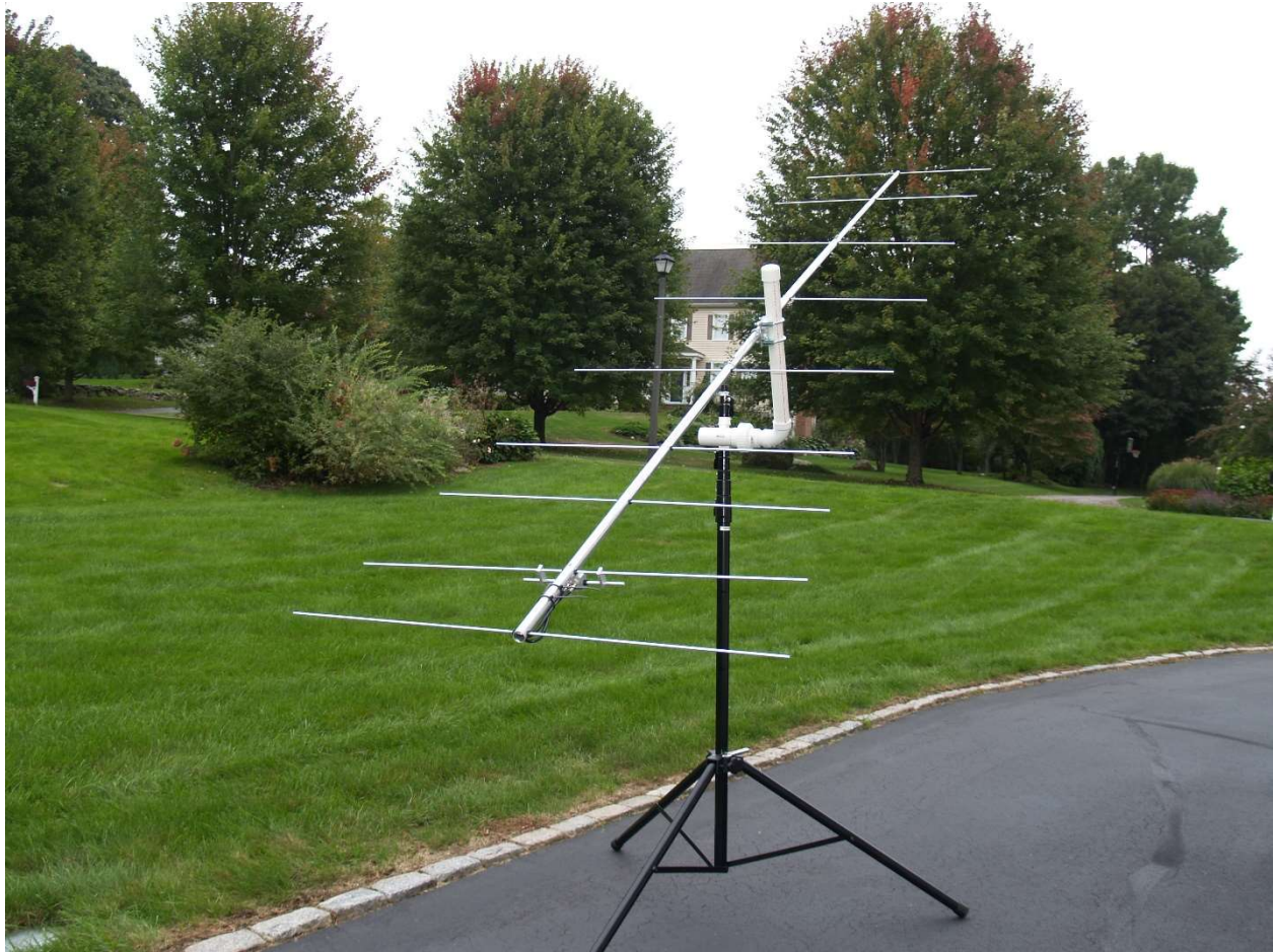
Figure 14. M 2 2M9SSB horizontally polarized Yagi-Uda antenna mounted on an MFJ-1918EX tripod at the KC1HTT EME site. [21]
