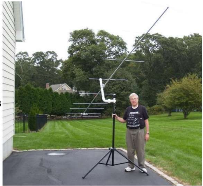
Figure 27. The KC1HTT amateur radio station parameters the night of January 19, 2019. Total antenna gain was calculated to include the antenna height, one wavelength above the ground and with an elevation angle of 15°. Ground gain contributed 2.46 dB to the total antenna gain. The power aperture (P*A) of this small EME station is +39.14 dBW. (Photo from 10/2018)
