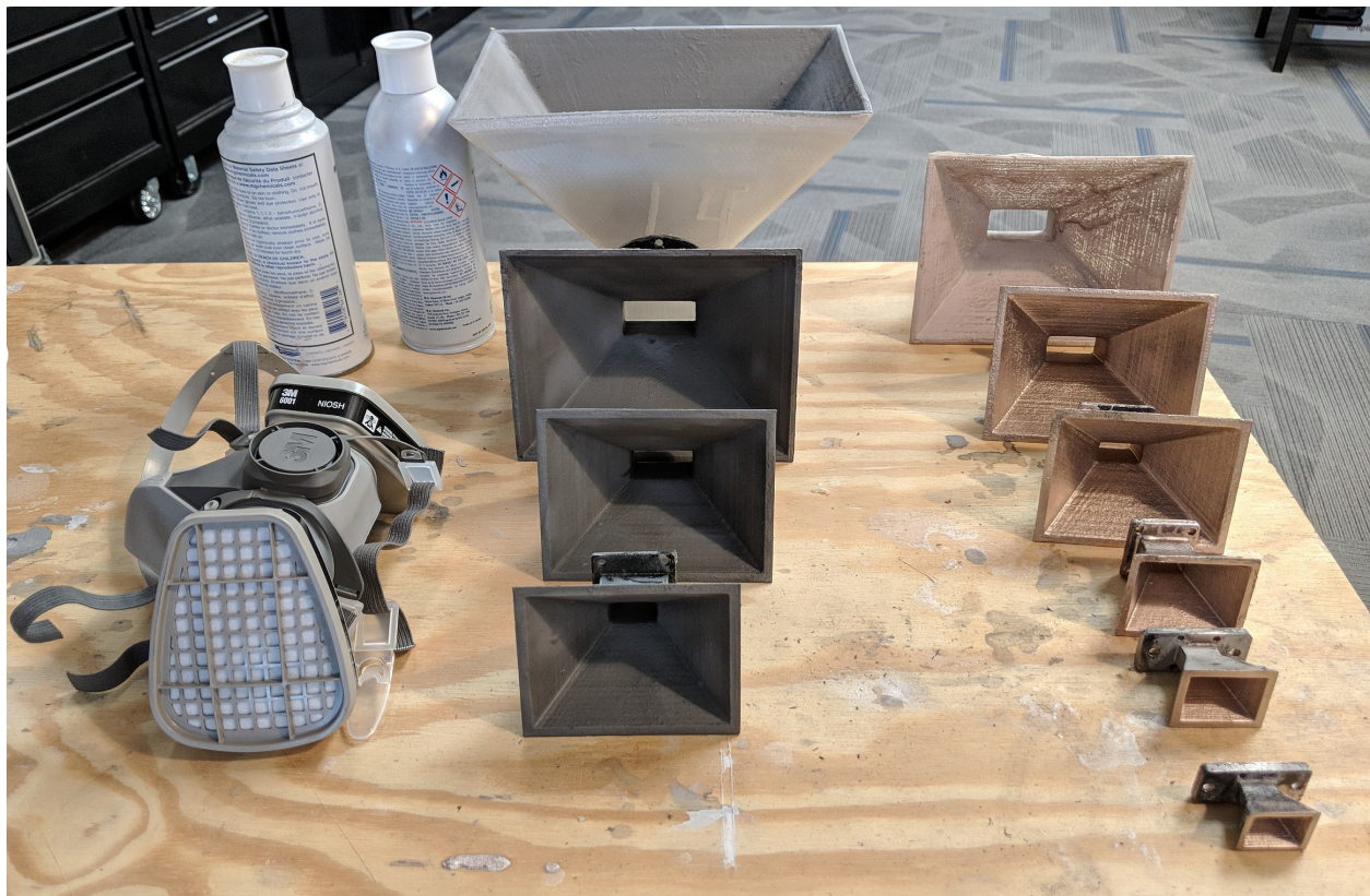
Figure 2: 3D Printed Horns Smallest K-Band to Largest S-Band
